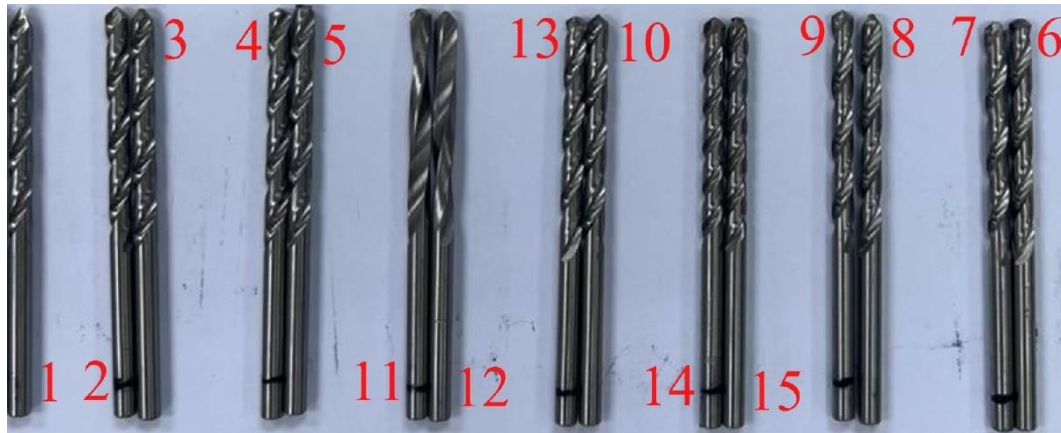
Fig. 6. Actual image of customized drill bits used in the study
