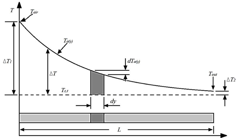
Fig. 7. Diagram of the heat transfer process within a GHE pipe [39]
