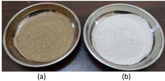
**Fig. 4.** Getting ready to put in the oven: (a) native soil and (b) bentonite
