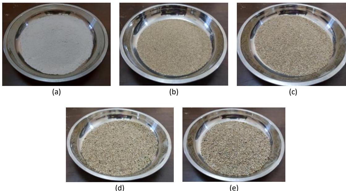
**Fig. 3.** Elements that used in this study which are (a) bentonite and four grain sizes of native soil: (b) 0.6-1.0mm, (c) 1.0-1.6mm, (d) 1.6-2.0mm and (e) 2.0-2.5mm
