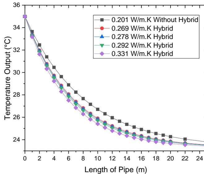
**Fig. 10.** Length of the pipe against air temperature for five thermal conductivity values
