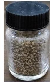
**Fig. 5.** Samples of hybrid soil that is a mix of native soil grain size 0.6-1.0mm and bentonite
