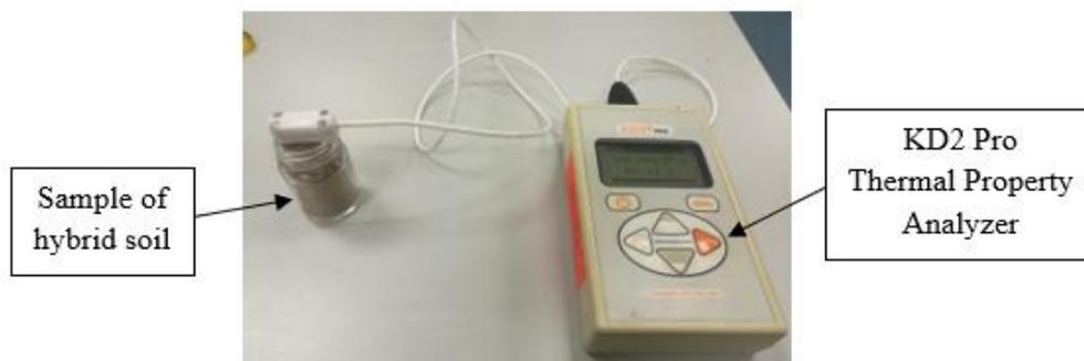
**Fig. 6.** The KD2 Pro Thermal Property Analyzer is used to measure thermal conductivity
