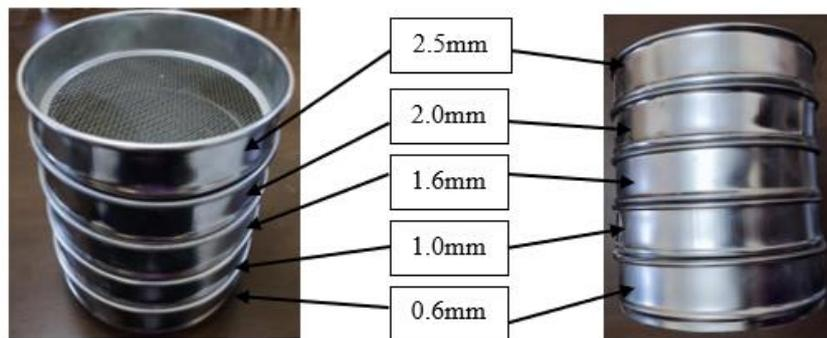
Fig. 2. Sieve in four different ranges
