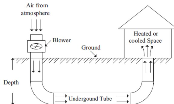
Fig. 1. Basic principle for open system GHE [17]
