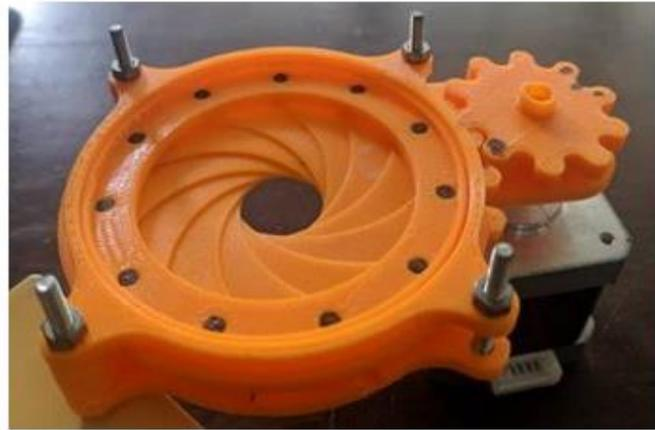
**Fig. 4.** The active air damper prototype
