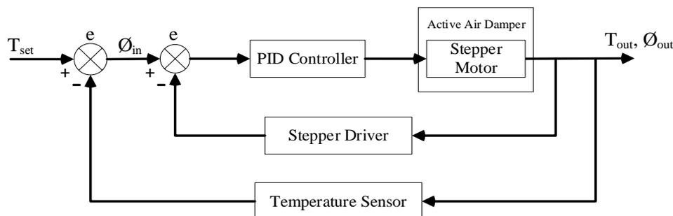
Fig. 7. The schematic diagram of the PID control system
