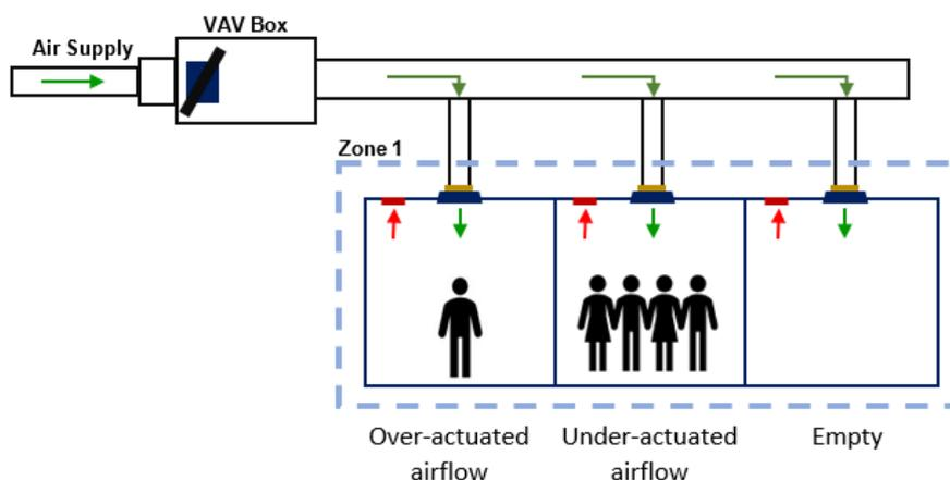
Fig. 1. The air flow distribution problems in VAV system
