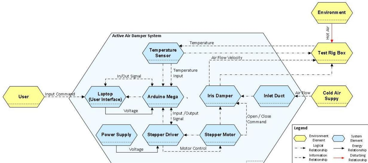
Fig. 6. The illustration of experimental analysis set-up
