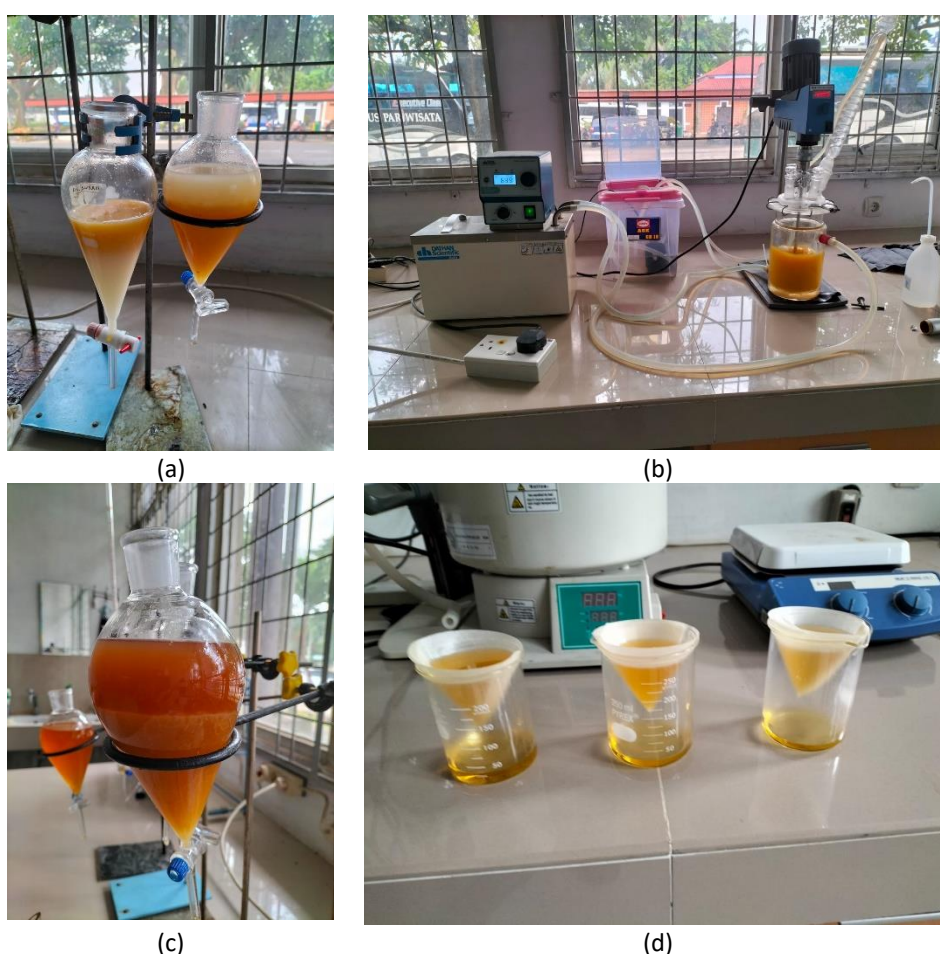
Fig. 1. RSB production process; (a) Degumming, (b) Esterification-Transesterification in Double jacket reactor, (c) deposition, (d) filtering
