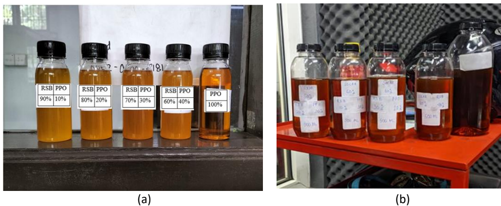
Fig. 3. Fuel samples for testing (a) physico-chemical properties, (b) Engine Performance
