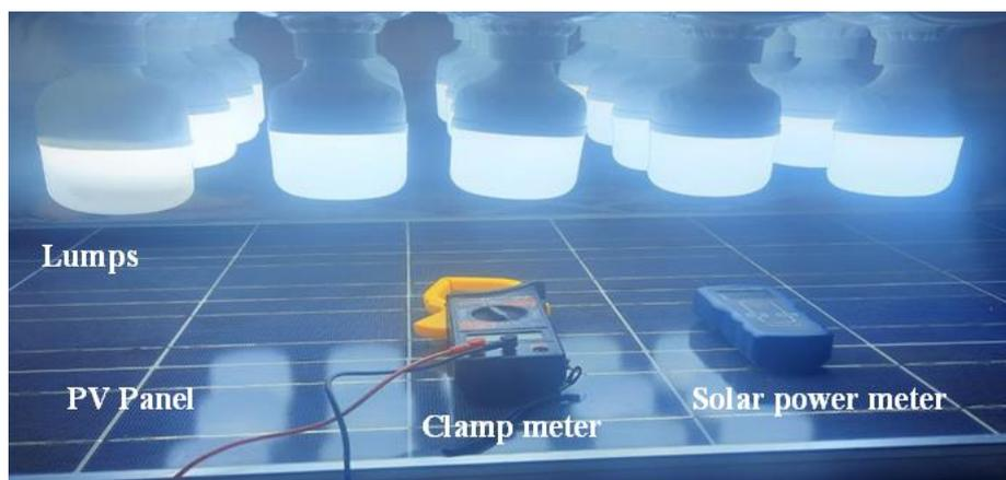
**Fig. 1.** Experimental set-up for the current study
