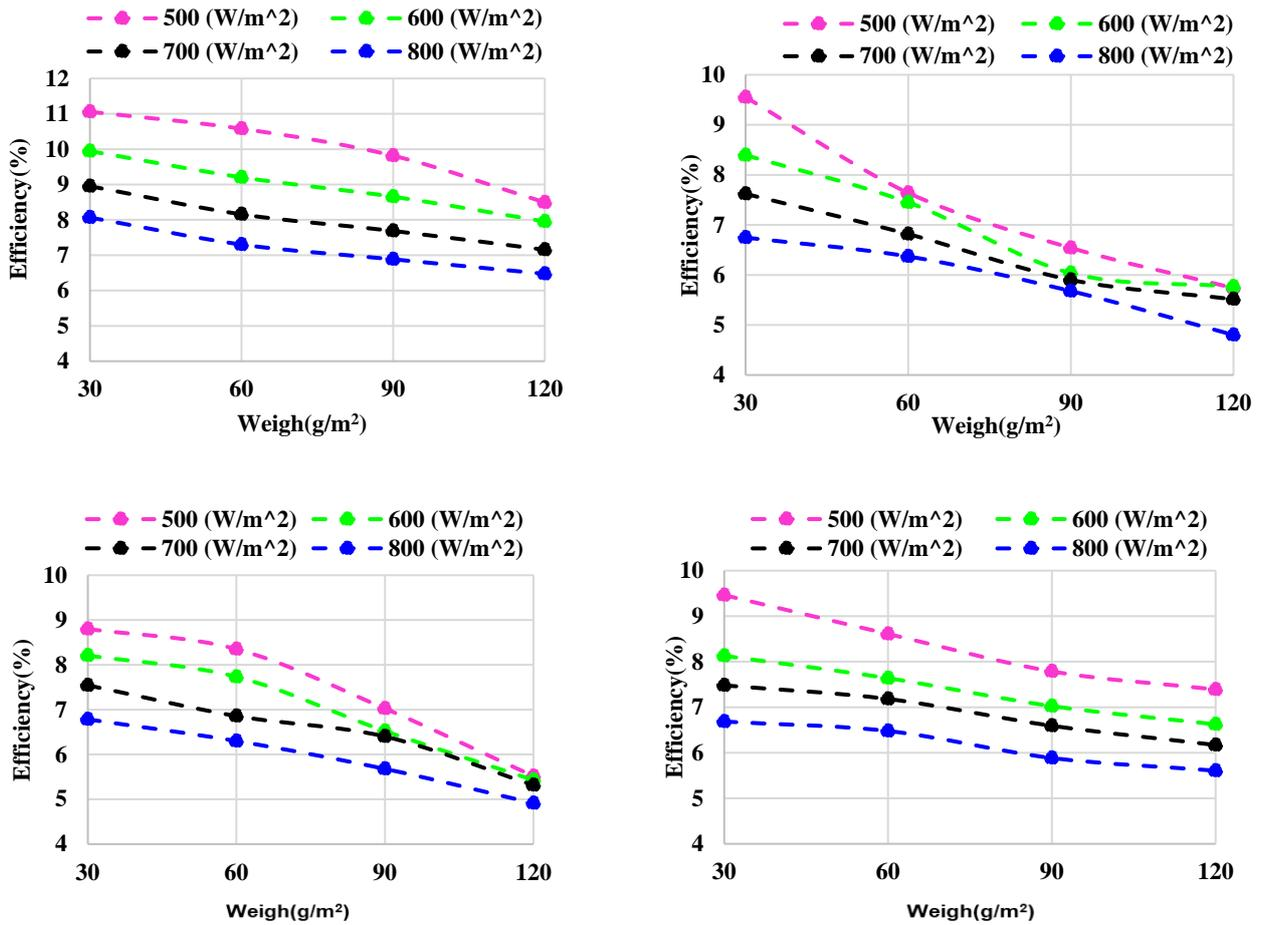
Fig. 4. The efficiency-weight responses of several dust kinds. The following are examples of powders: chalk, brick, sand, and coal
