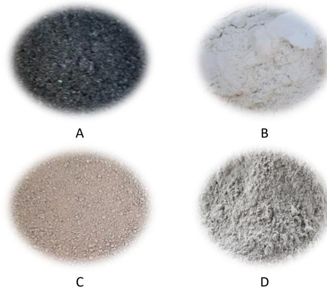
**Fig. 2.** Dust samples for current study: A. Chalk powder, B. Brick powder, C Sand, D. Coal powder
