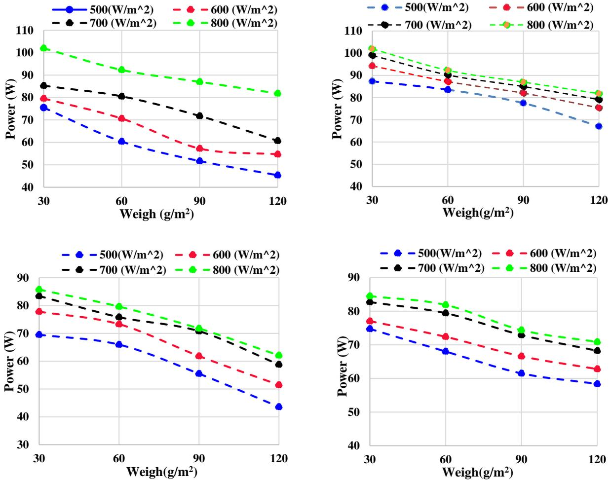
**Fig. 3.** The power-weight responses of several dust kinds. The following are examples of powders: chalk, brick, sand, and coal
