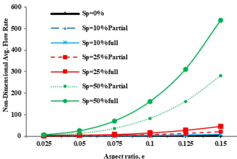
**Fig. 5.** Non-dimensional cyclic average oil flow rate between piston ring and cylinder liner
