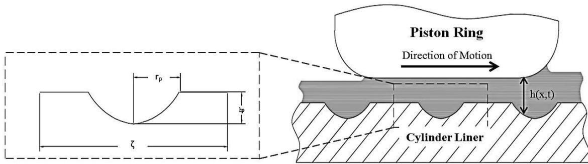
**Fig. 3.** Schematic drawing of a single surface cell containing one oil groove
