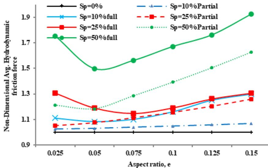
**Fig. 6.** Effect of grooves aspect ratio on non-dimensional cyclic average hydrodynamic friction force
