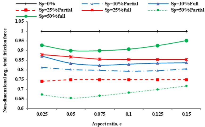
**Fig. 7.** Effect of grooves aspect ratio on non-dimensional cyclic average asperity contact friction force
