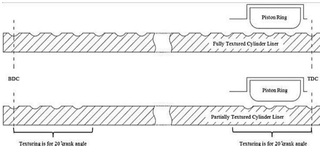
**Fig. 2.** Schematic cross-section of fully and partially cylinder liner
