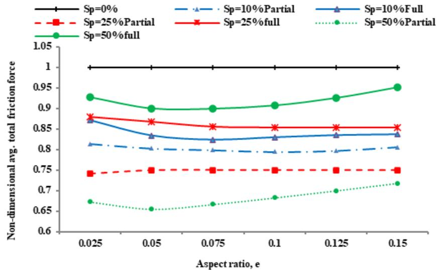
**Fig. 8.** Effect of grooves aspect ratio on non-dimensional cyclic average total friction force
