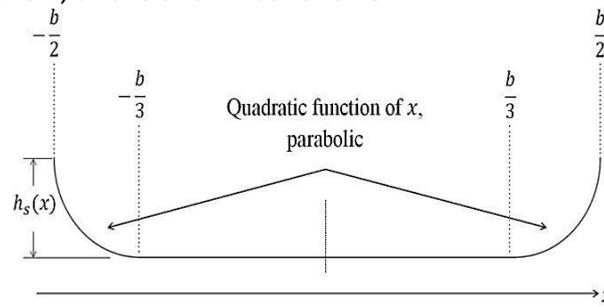
Fig. 1. Details of piston ring face profile textured
