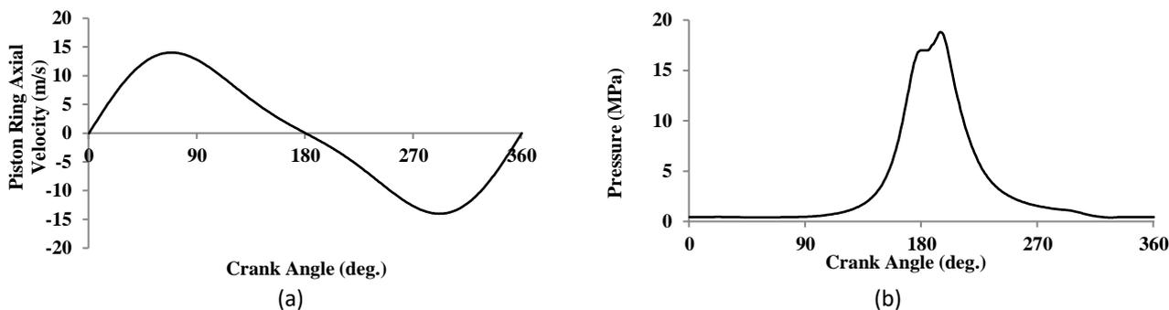
**Fig. 4.** Dynamic parameters of piston ring (a) Piston ring linear velocity (b) Combustion chamber gas pressure
