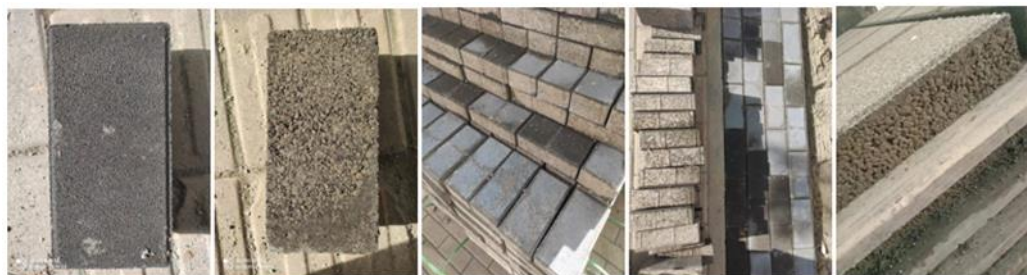
Fig. 1. Porous paver and its construction
