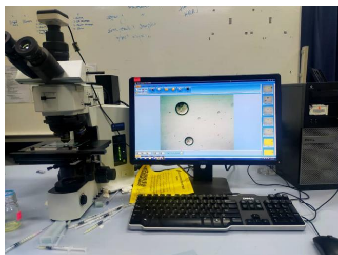
Fig. 5. Polarizing microscope with 50x magnifications
