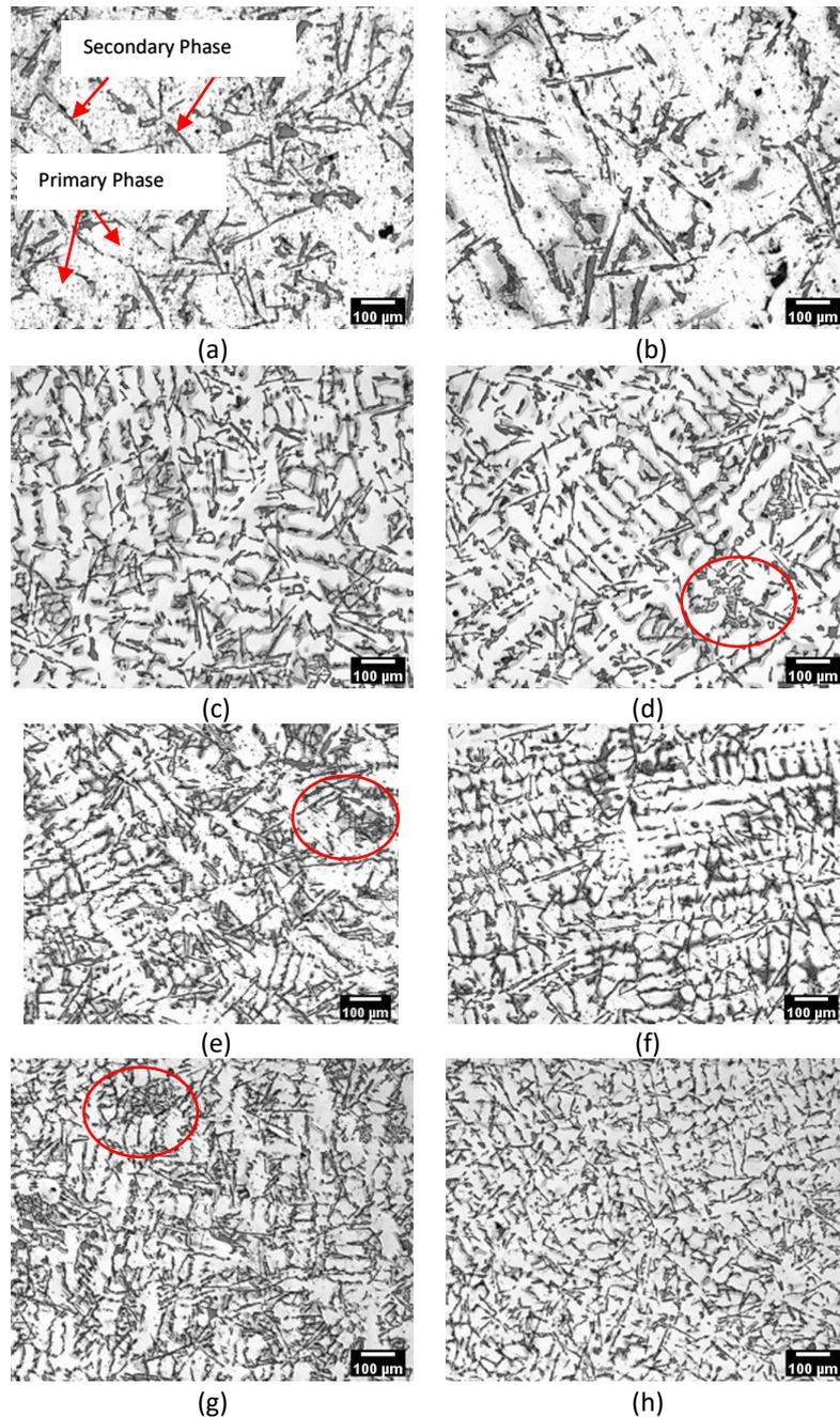
**Fig. 4.** Microstructure evolution of the solidified material at the crucible centre (left) and at the crucible wall (right) with cooling rate of (a), (b) 0.16 °C/s, (c), (d) 1.0 °C/s, (e), (f) 1.3 °C/s, and (g), (h) 1.9 °C/s. (5x magnification)
