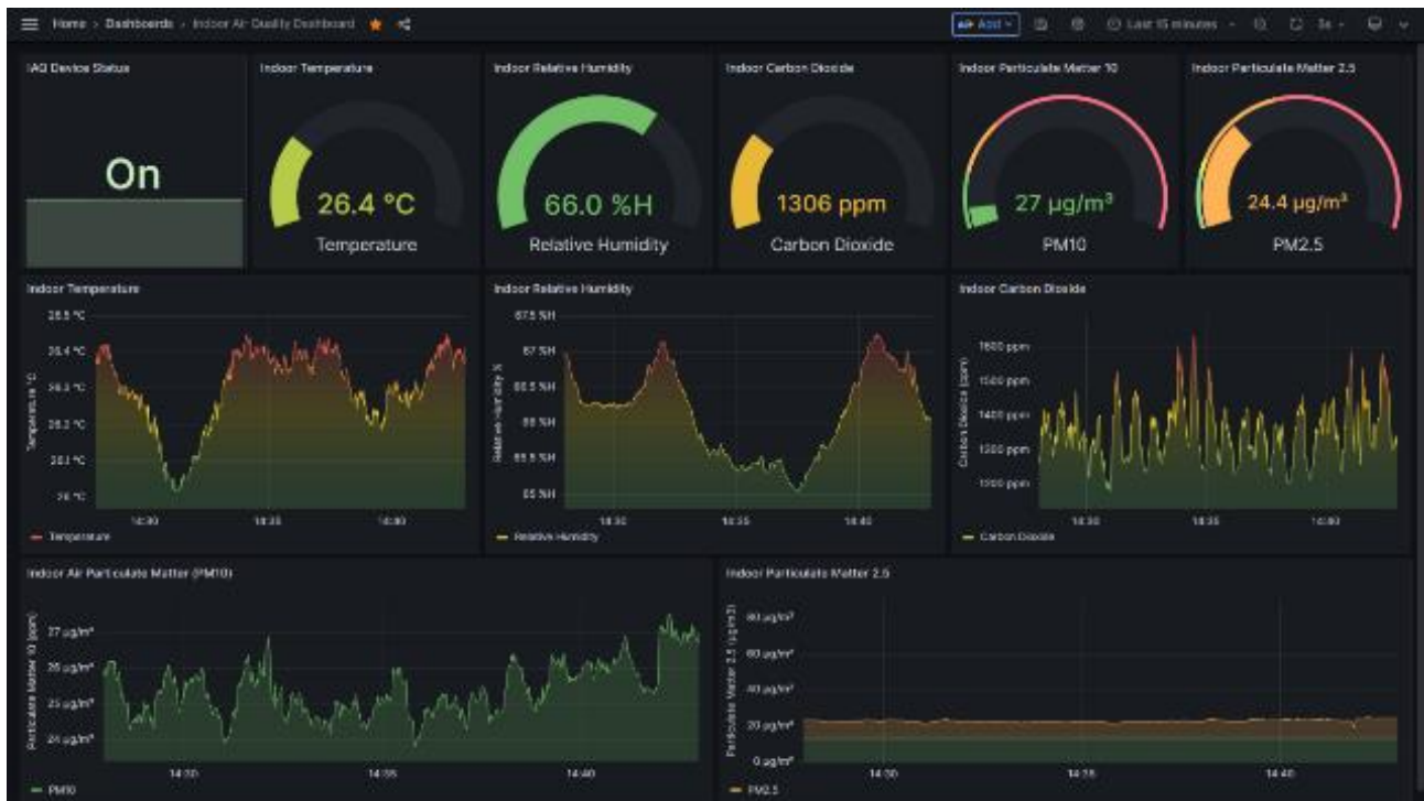
Fig. 5. IAQ Remote Monitoring Dashboard displaying Real-Time Data by using Grafana software
