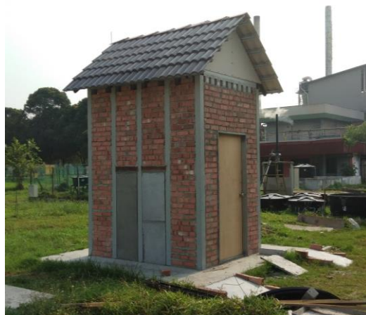
Fig. 2. Model house with a wall panel of normal and fine coconut shell concrete use in this study
