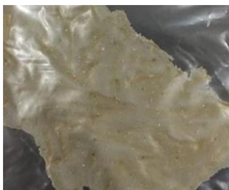
Fig. 2. Dried bioplastic from sweet potato starch studies above
