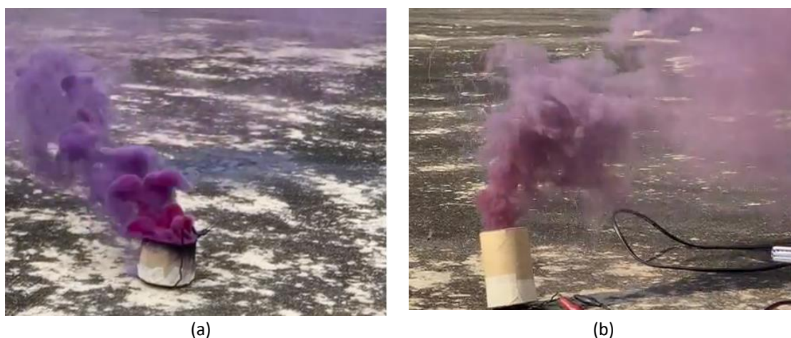
Fig. 8. Smoke Emission of (a) KClO_3 -based formulation and (b) KNO_3 -based formulation at 30 seconds
