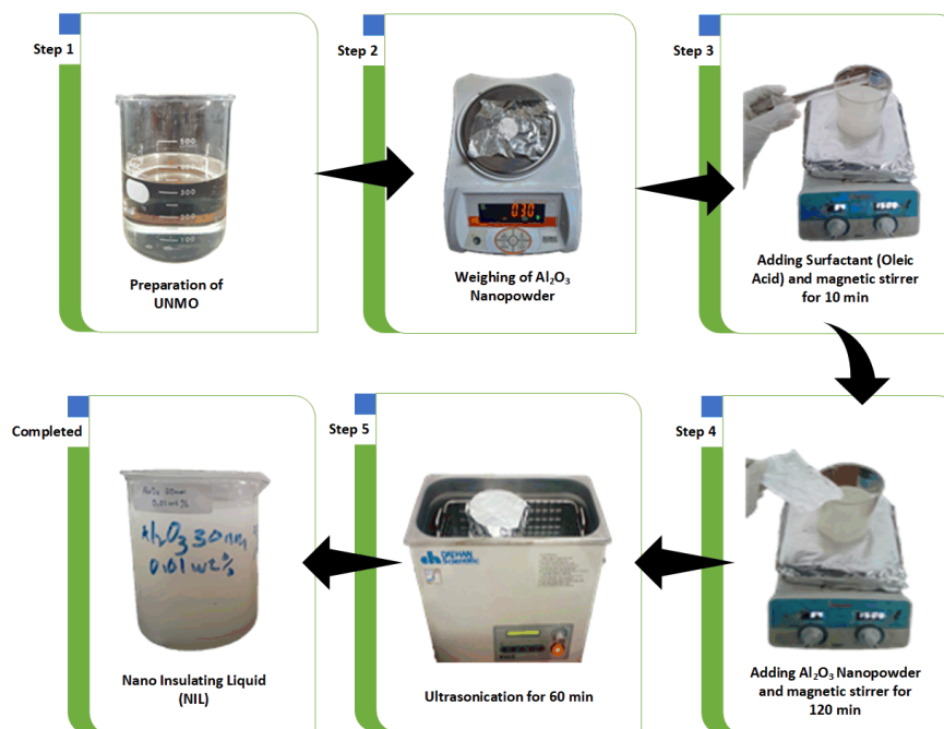
Fig. 1. Preparation of nano insulating liquid
