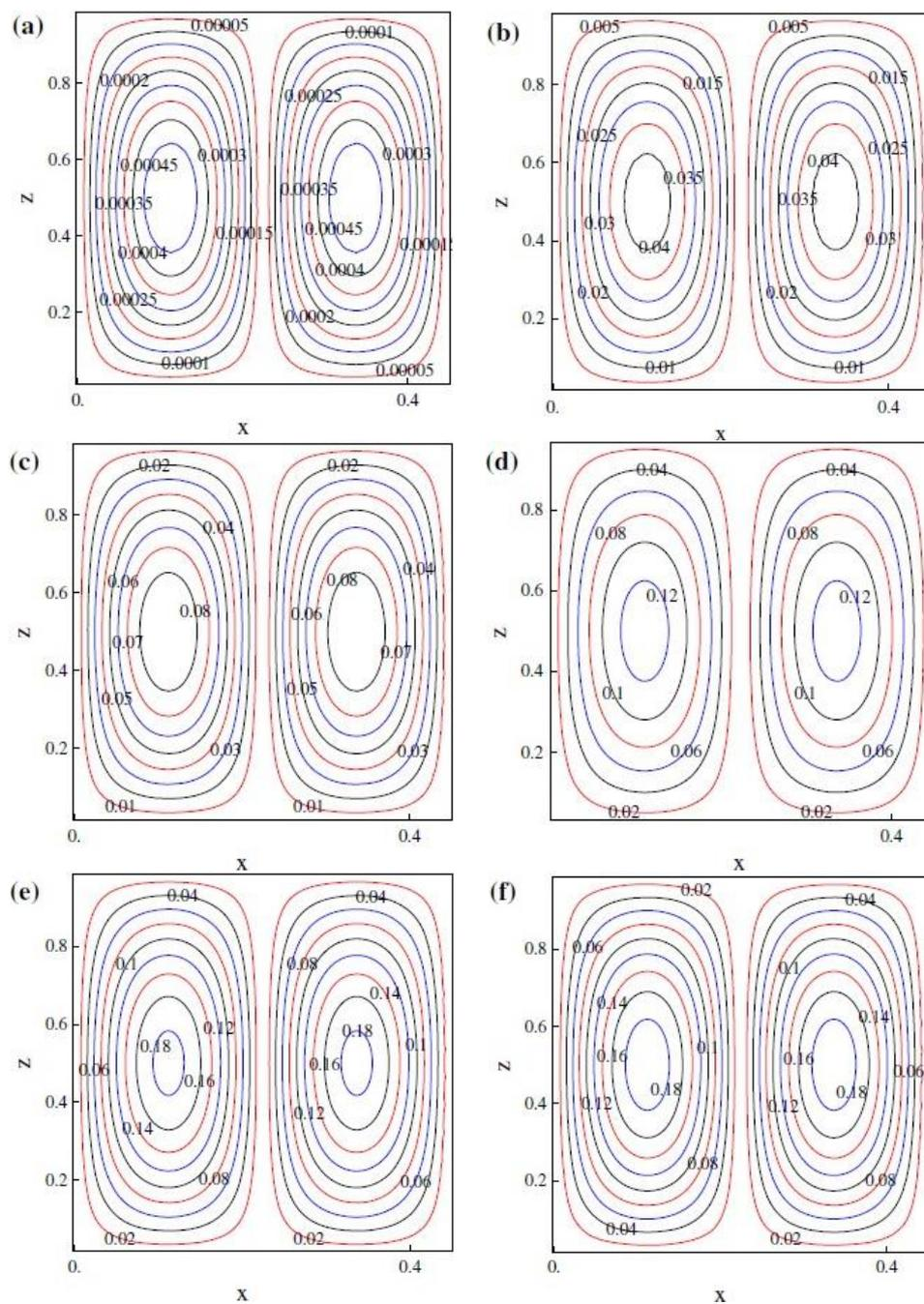
**Fig. 11.** Streamlines for various values of times (a)  $s = 0.0$ , (b)  $s = 0.12$ , (c)  $s = 0.14$ , (d)  $s = 0.15$ , (e)  $s = 0.16$ , (f)  $s = 0.17$
