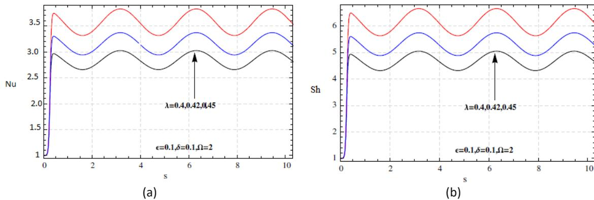
Fig. 6. Effect of  $\lambda$  on (a)  $Nu$ , and (b)  $Sh$ , for fixed values of other parameters
