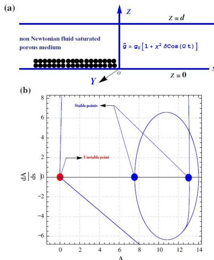
**Fig. 1.** (a) Physical configuration of the problem, (b) Supercritical pitchfork bifurcation diagram
