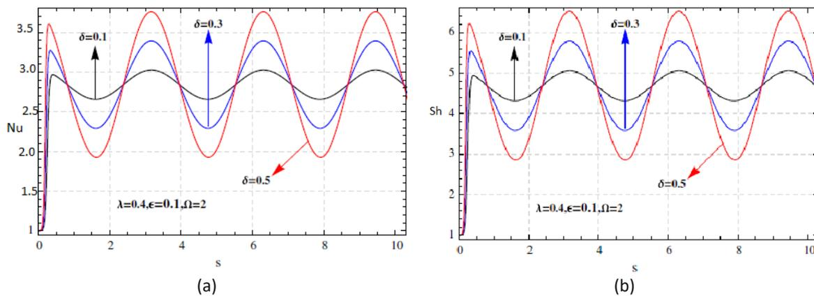
Fig. 8. Effect of  $\delta$  on (a) Nu, and (b) Sh, for fixed values of other parameters
