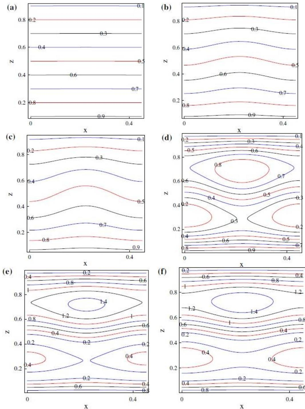
**Fig. 12.** Isotherms for various values of times (a)  $s = 0.0$ , (b)  $s = 0.12$ , (c)  $s = 0.14$ , (d)  $s = 0.15$ , (e)  $s = 0.16$ , (f)  $s = 0.17$
