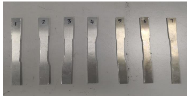
Fig. 3. Samples post-cutting for tensile testing
