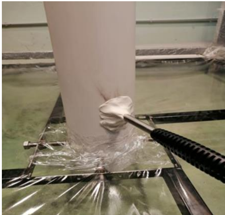
Fig. 5. The position of anemometer for velocity measurement
