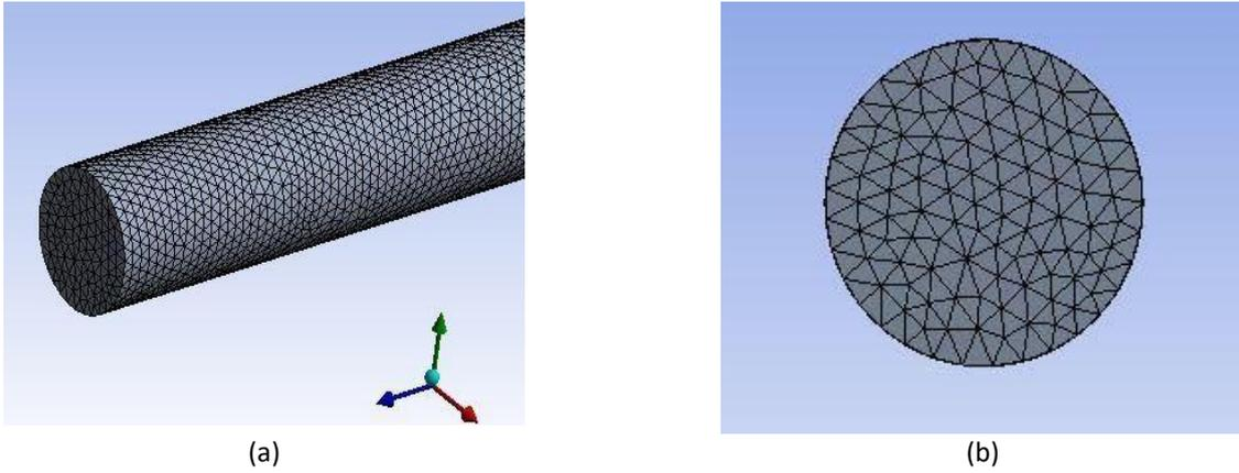
Fig. 2. (a) Mesh elements along horizontal pipe (b) C.S. view of horizontal pipe
