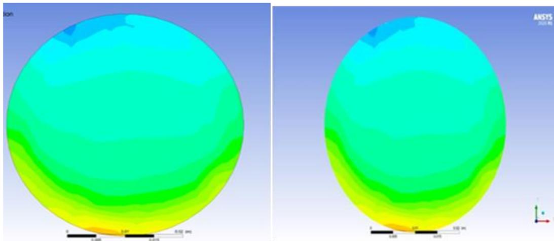
**Fig. 6.** Solid volume fraction contour of fly ash at 65% concentration at velocity 1m/s and 3m/s in horizontal pipe
