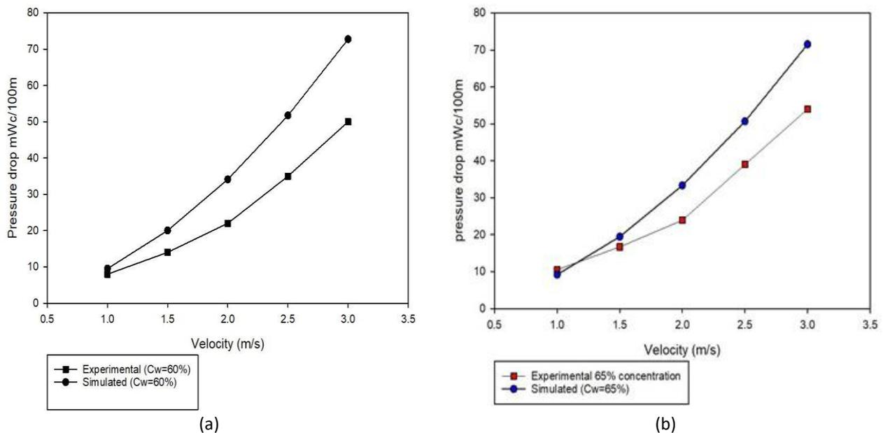
Fig. 4. Pressure drop Vs velocity at a solid concentration (a) 60% and (b) 65% by weight in horizontal pipe
