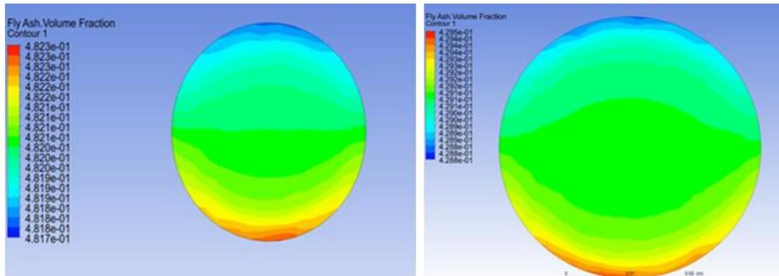
**Fig. 5.** Solid volume fraction contour of fly ash at 60% concentration at velocity 1m/s and 3m/s in horizontal pipe
