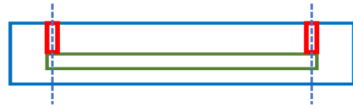
Fig. 2. Longitudinal view of microfluidic chip with constant depth microchannel
