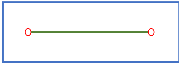
Fig. 1. Microfluidic chip top view (Green-microchannel, Red-ports)
