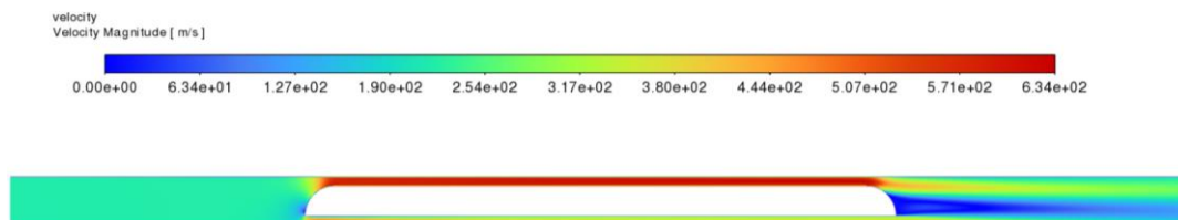
Fig. 7. Semicircular Capsule model: Velocity contour(Max. Velocity = 634 m/s)
