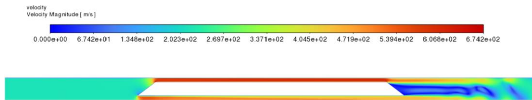
Fig. 5. Linear Capsule model: Velocity contour(Max. Velocity = 674 m/s)
