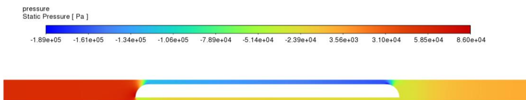
Fig. 8. Semicircular Capsule model: Pressure contour(Max. Pressure = 8.60 \times 10^4 Pa)
