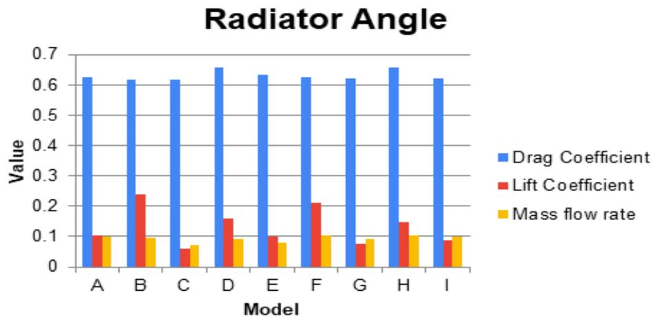
**Fig. 4.** Drag coefficient, lift coefficient and mass flow rate of different radiator angles
