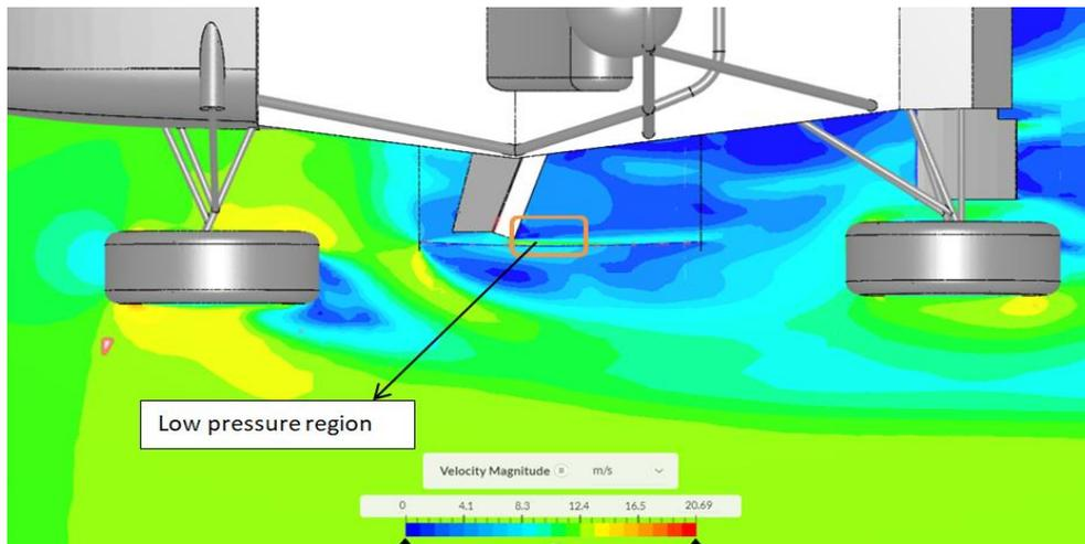
**Fig. 11.** Velocity contour of low-pressure region at the side end of the radiator
