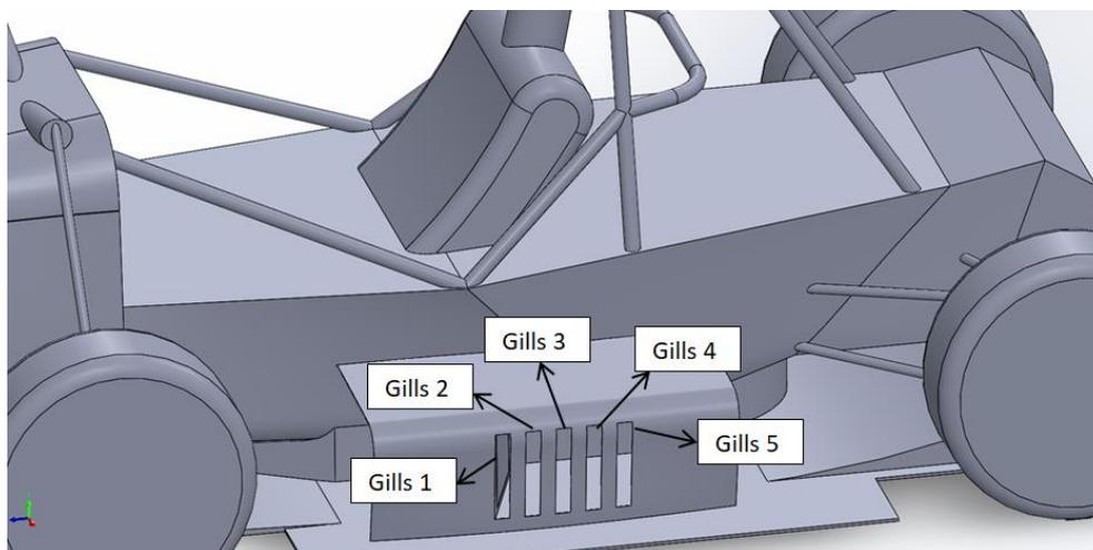
**Fig. 12.** CAD model of sidepod gills
