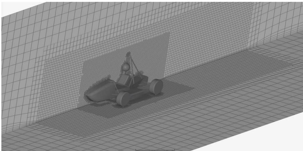
**Fig. 1.** Computational domain with the generated mesh
