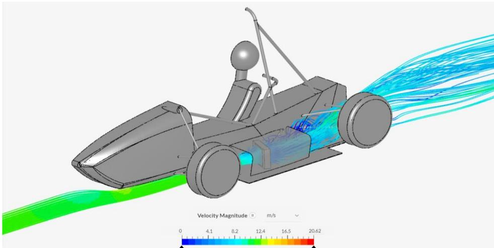
**Fig. 8.** Velocity streamlines passing through the radiator core of model LL
