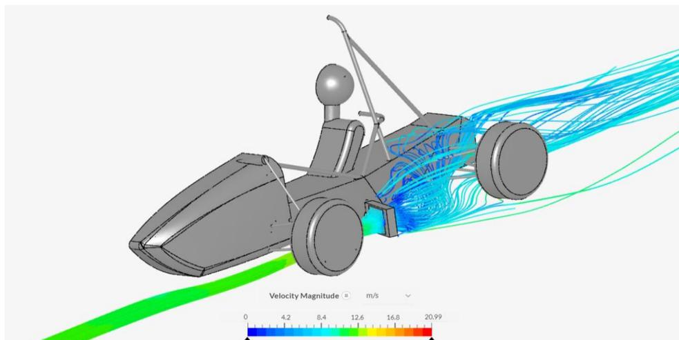
**Fig. 5.** Velocity streamlines passing through the radiator core of model F
