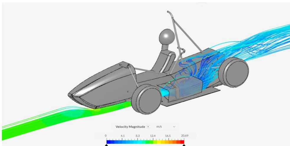
**Fig. 10.** Velocity streamlines passing through the radiator core of case Q
