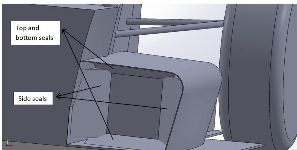
**Fig. 9.** CAD model of radiator seals
