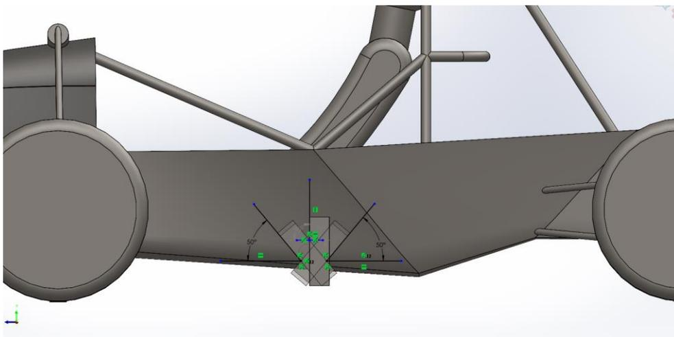
**Fig. 3.** 50- and 90-degree radiator angles from side view
