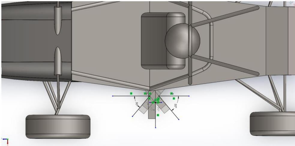
**Fig. 2.** 50- and 90-degree radiator angles from top view
