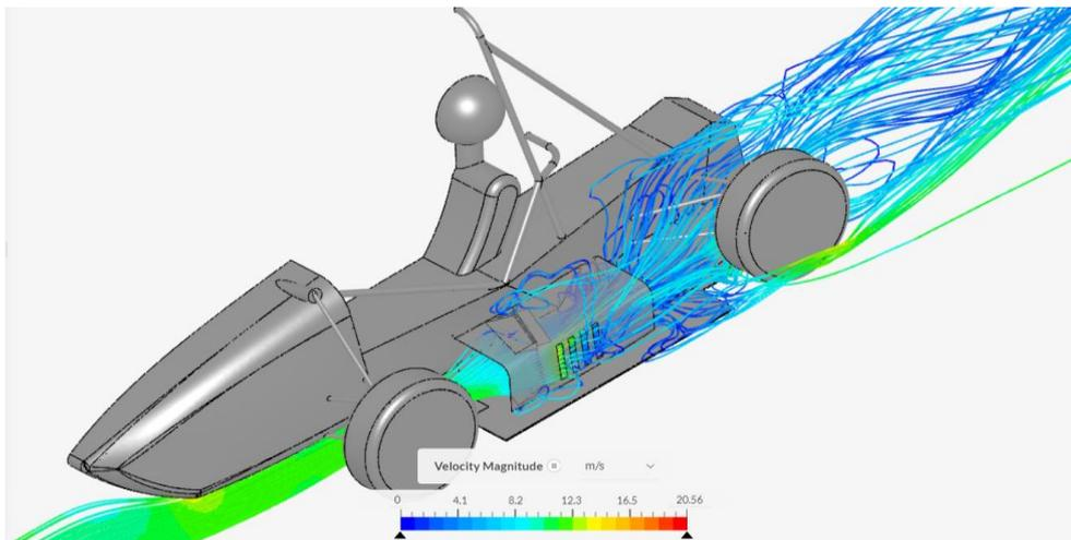
**Fig. 13.** Velocity streamlines passing through radiator core of gills 4 model
