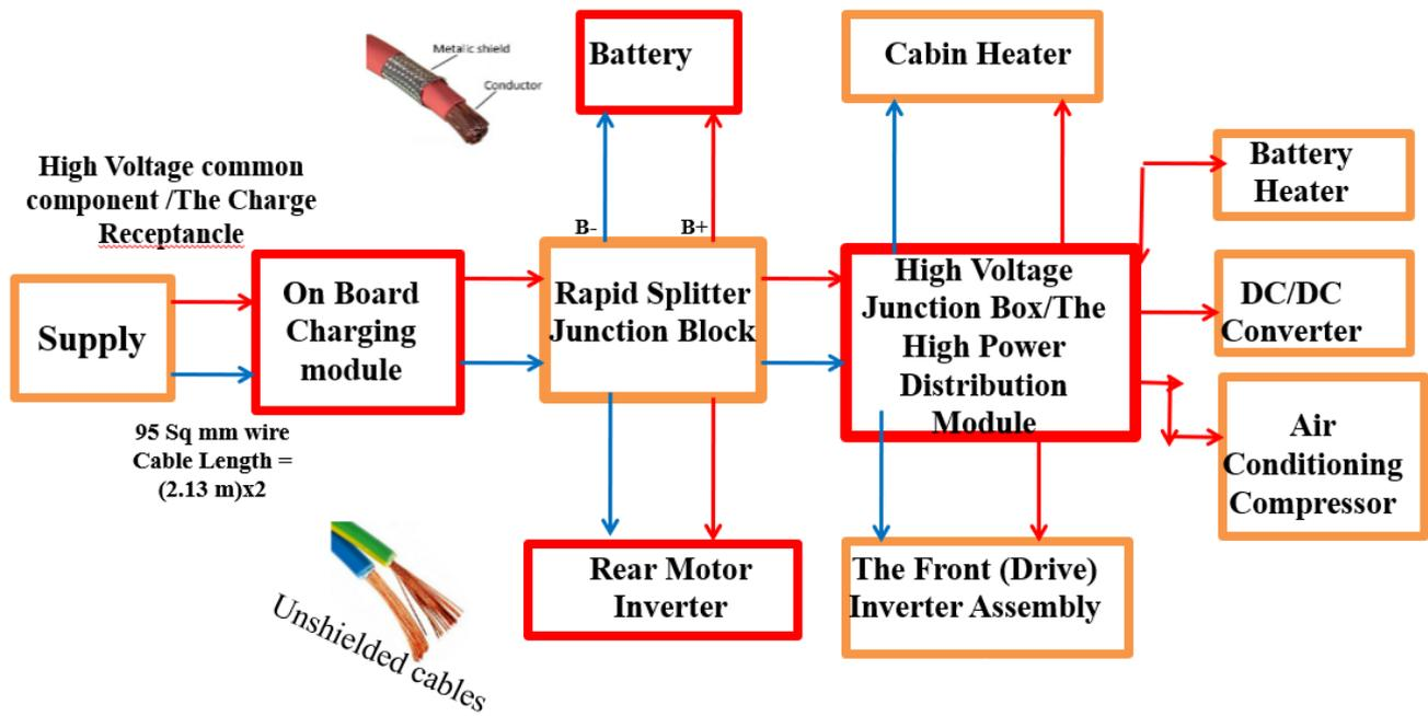
Fig. 1. High voltage cabling network of EV
