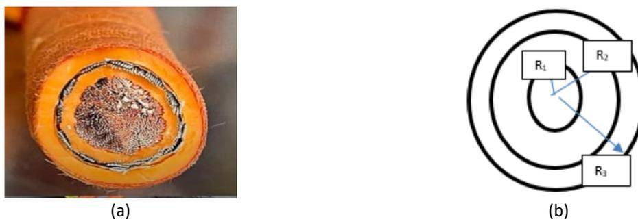
Fig. 2. Practical EV Cabling layers (a) Cross-section view of EV cable [19] (b) Geometrical structure of cable
