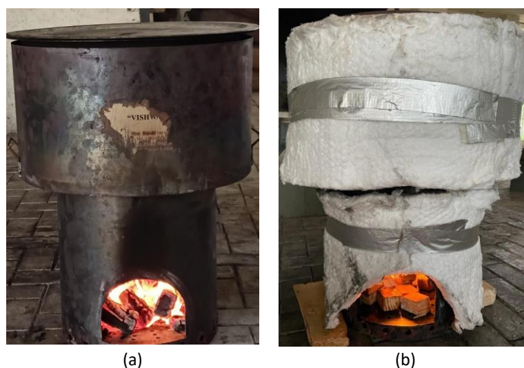
Fig. 5. Images of the cookstove during laboratory tests, (a) cookstove without insulation, (b) cookstove with insulation
