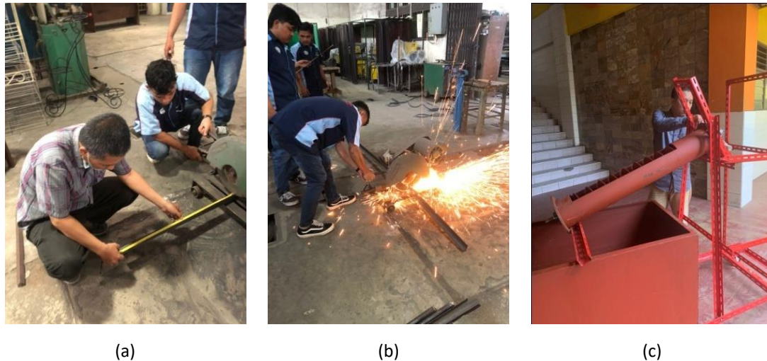
Fig. 2. Photo documentation of the manufacturing process of the picohydro technology test equipment (a) Measurement and preparation of the cutting process (b) Component cutting process (c) Assembly test tool
