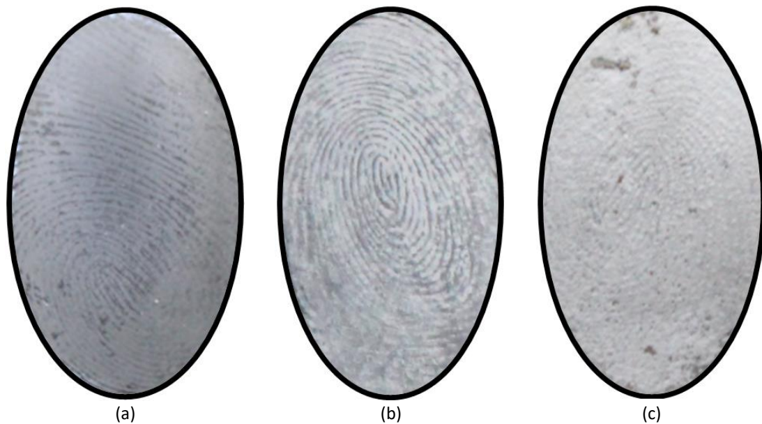
Fig. 6. Latent fingerprints (a) before and after cyanoacrylate exposure for (b) 30 minutes and (b) 60 minutes
