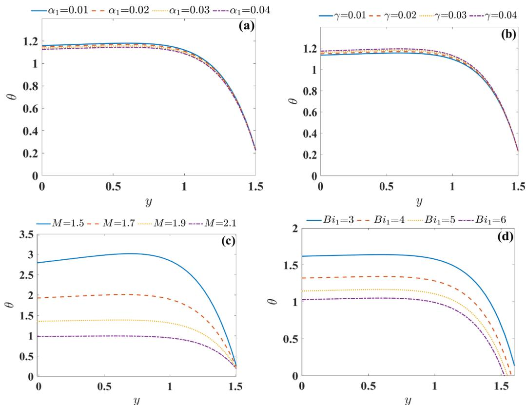
**Fig. 4.** Temperature graphs for distinctive values of (a) variable viscosity, (b) variable thermal conductivity, (c) magnetic parameters (d) Biot number
