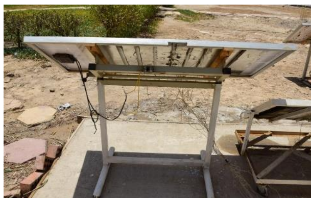
Fig. 1. PV-Aluminium Finned Wall module structure
