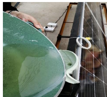
Fig. 6. Pouring paraffin wax into the aluminum container
