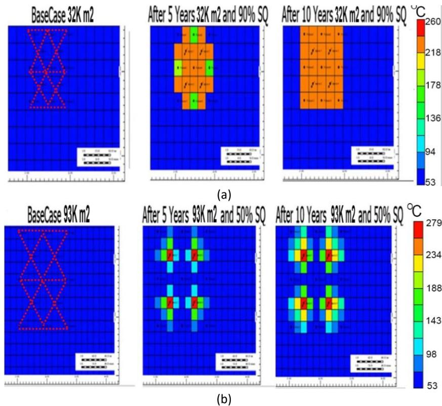
**Fig. 6.** Heat transfer in clean (homogenous) sand before and after steamflood using (a) 32,374.90 m<sup>2</sup> with 90% steam quality and (b) 93,077.7 m<sup>2</sup> with 50% steam quality
