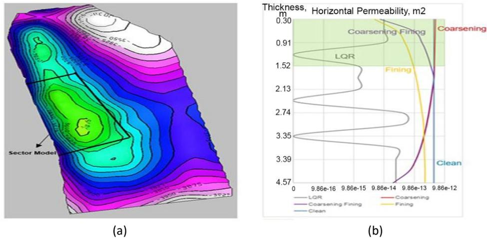
**Fig. 1.** (a) Contour map and (b) Horizontal permeability log of the XYZ field
