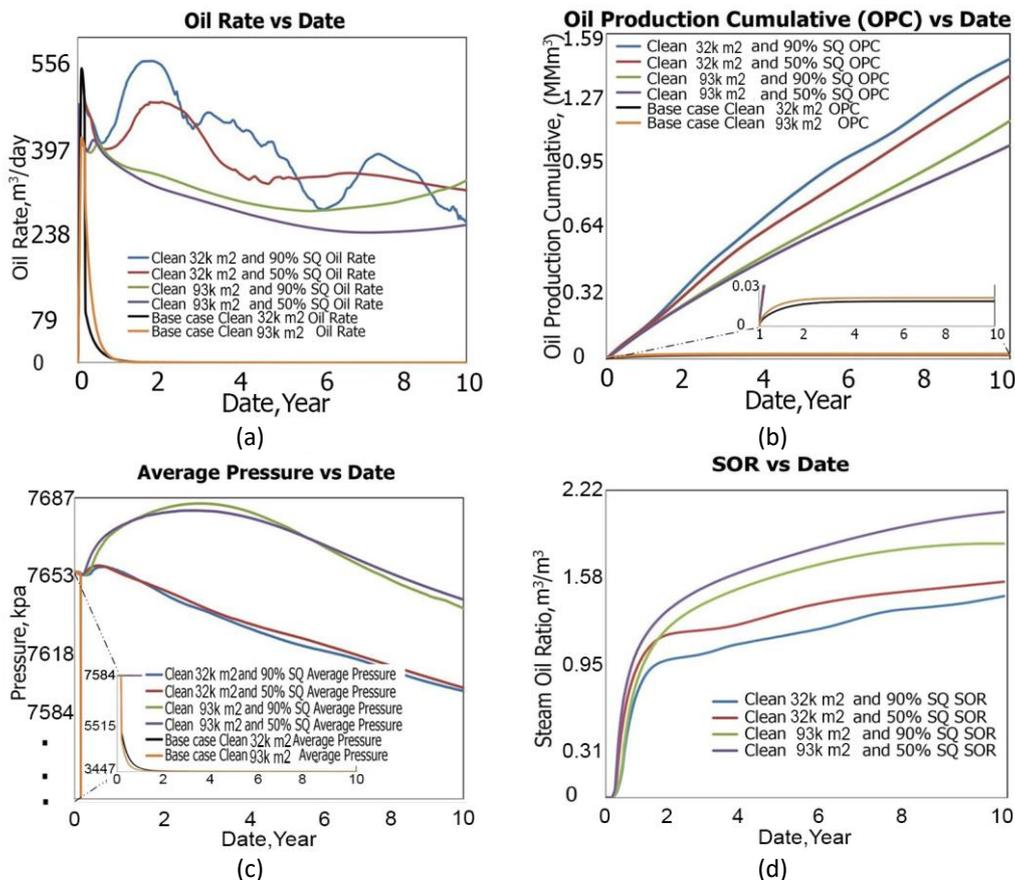
**Fig. 5.** (a) oil rate, (b) OPC, (c) average pressure, (d) SOR performance in clean (homogenous) sand before and after steamflood
