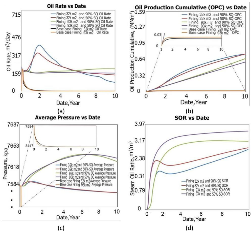
**Fig. 7.** (a) oil rate, (b) OPC, (c) average pressure, (d) SOR performance in fining sand before and after steamflood
