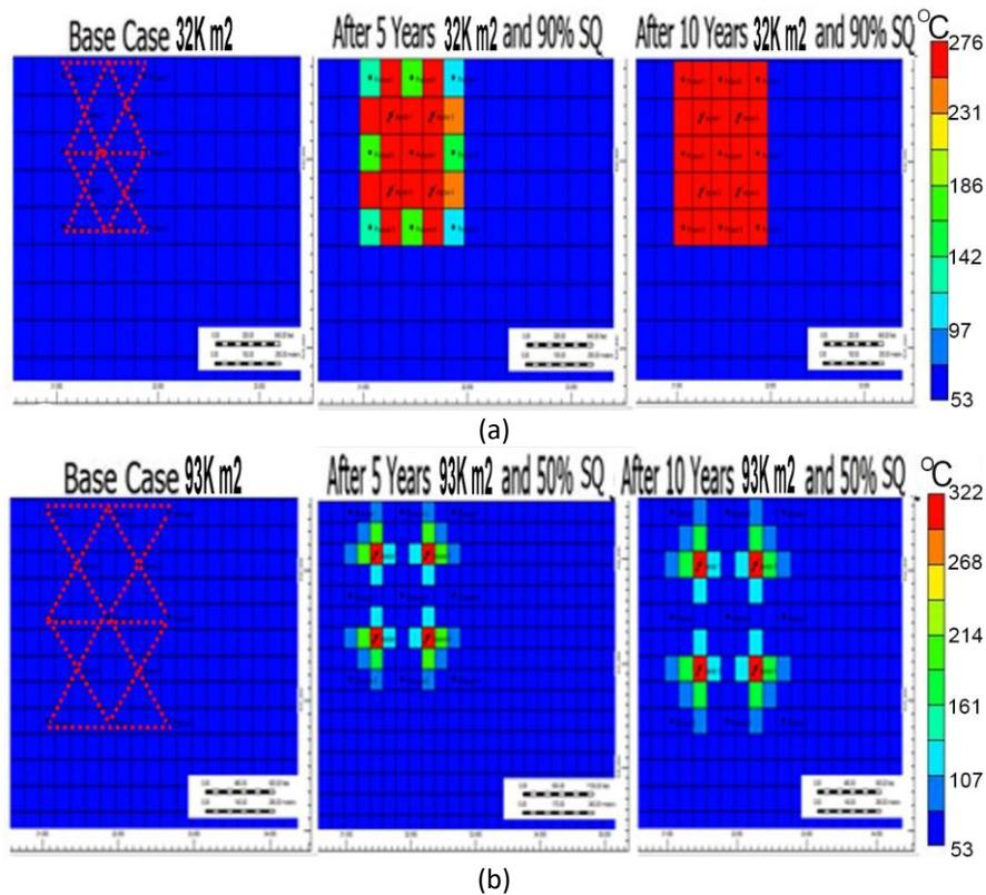
**Fig. 8.** Heat transfer in fining sand before and after steamflood using (a) 32,374.90 m<sup>2</sup> with 90% steam quality and (b) 93,077.7 m<sup>2</sup> with 50% steam quality
