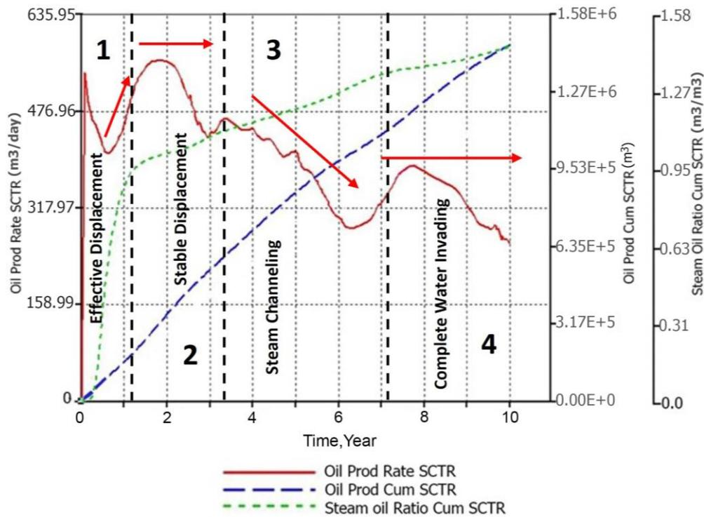
**Fig. 4.** Clean sand performance with 32,374.90 m<sup>2</sup> of well spacing and 90% steam quality
