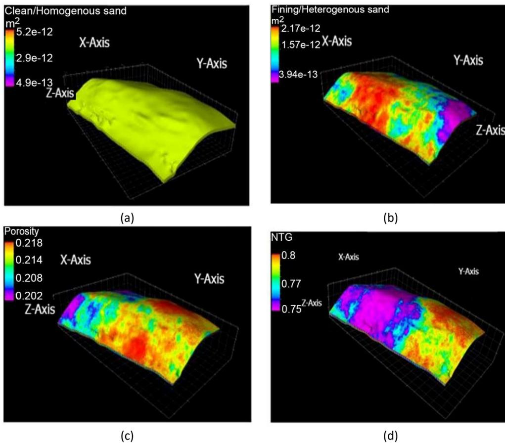
**Fig. 2.** Distribution of different sand types (a) clean (homogenous), (b) fining (heterogenous) and (c) porosity, and (d) NTG of the reservoir model
