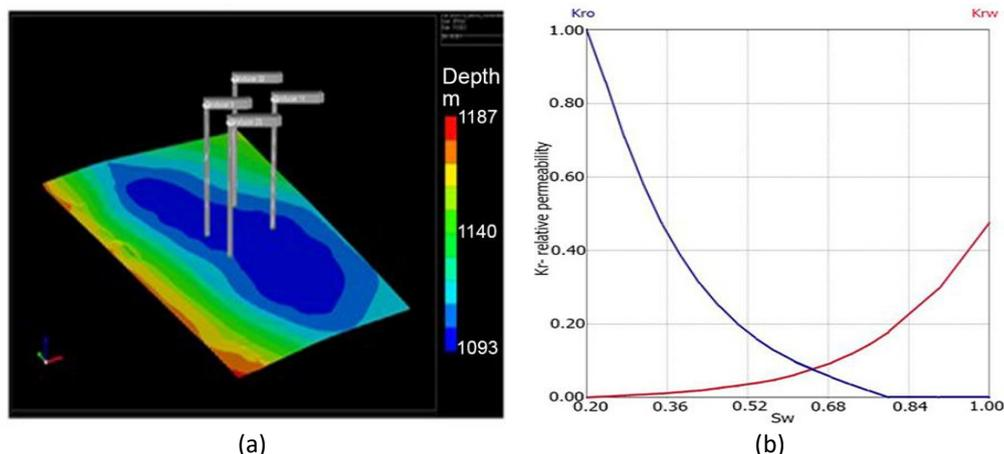
**Fig. 3.** (a) the distribution of wells, and (b) the relative permeability data in the XYZ field
