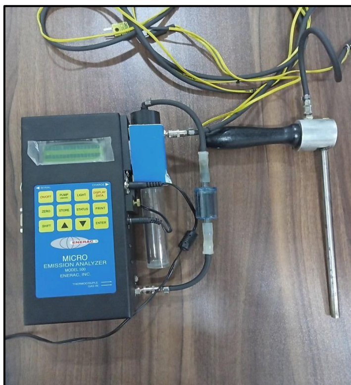
Fig. 3. Micro emission analyzer model 500 (Enerac)
