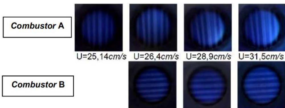
Fig. 6. Visualization of combustor hexane flames A and B, at \phi = 0.87
