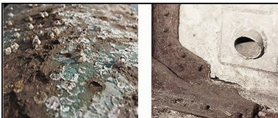
Fig. 2. Corroded Surfaces of Machine Parts
