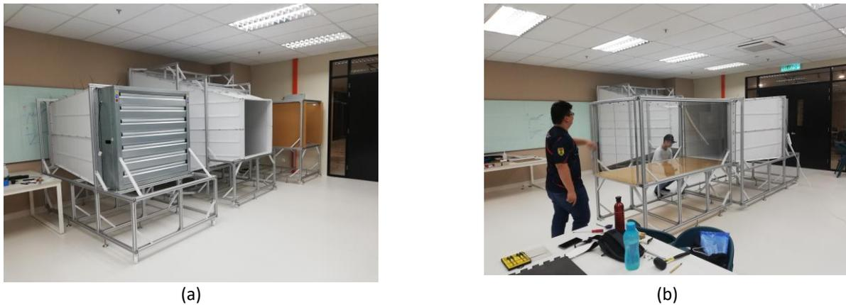
**Fig. 8.** (a) The modular form of the wind tunnel that parks at the corner of the lab for space saving (b) Assembly work of the tunnel
