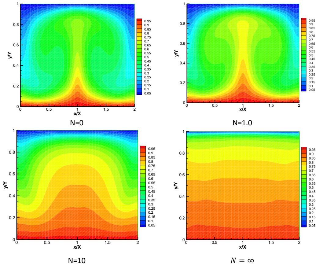
**Fig. 7.** Dimensionless steady state (SS) isotherms  $Ra = 510^4$ ,  $\omega = 0$  and  $Pr = 0.71$
