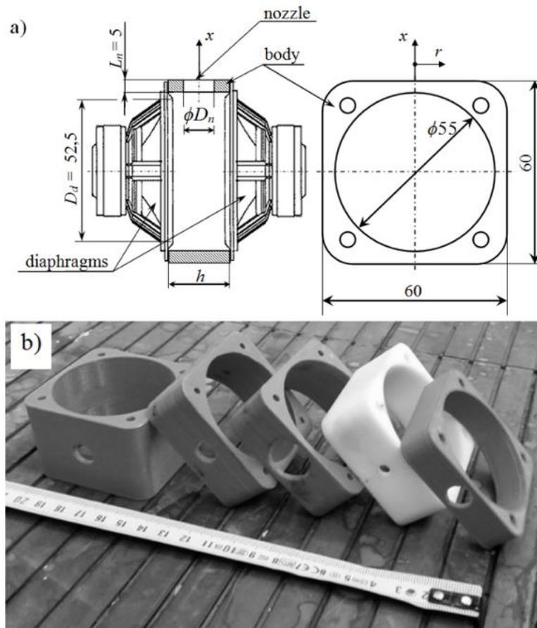
**Fig. 1.** (a) Schematic of the studied jet actuator; (b) Actuator photo [41]
