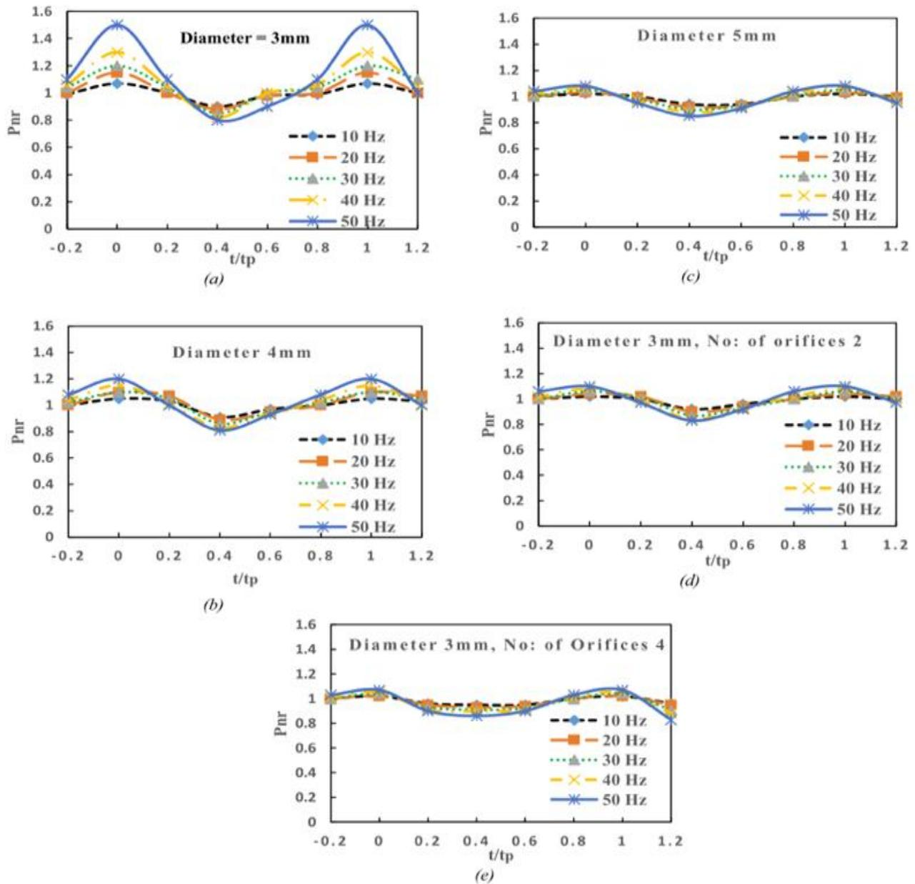
**Fig. 2.** Time history of cylinder pressure for different frequencies, (a) orifice diameter = 3 mm, (b) orifice diameter = 4 mm, (c) orifice diameter = 5 mm, (d) orifice diameter = 3 mm and number of orifices = 2, (e) orifice diameter = 3 mm and number of orifices = 4. [25]
