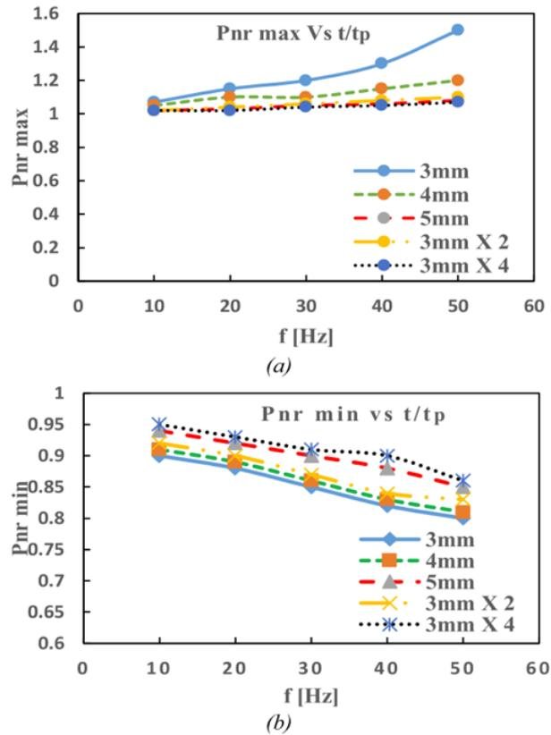
**Fig. 3.** The highest (a) and lowest (b) normalized cylinder pressures throughout the course of a cycle are displayed versus the actuation frequency [25]
