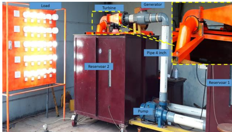
Fig. 1. The arrangement of the turbine apparatus
