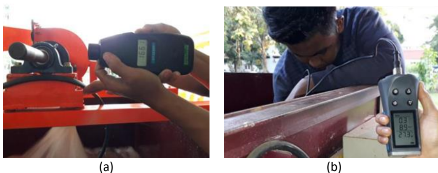
Fig. 2. Methods for rotations and flow mensuration. (a) Rotation (b) Flow rate
