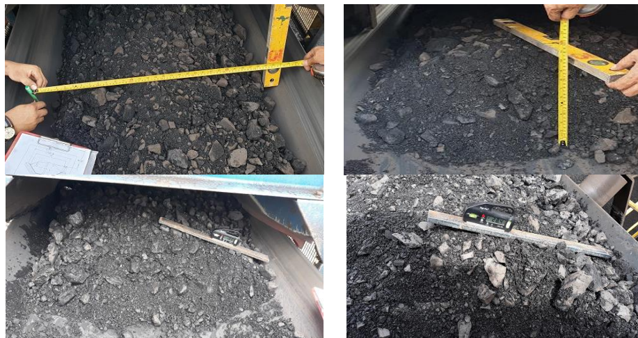
Fig. 6. Measuring coal pattern on the belt
