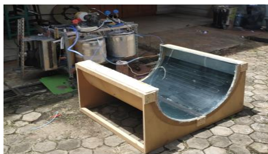
Fig. 4. Parabolic collector application to ORC
