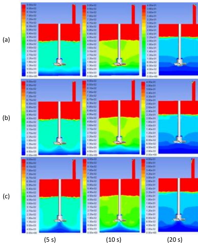
**Fig. 11.** Contour of biogas volume fraction at  $t = 20$ s. (a) 46 rpm, (b) 81 rpm and (c) 165 rpm
