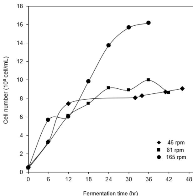
**Fig. 8.** Effect of stirring intensity on cell concentration in hydrogen fermentation by *E. aerogenes* NBRC 13534
