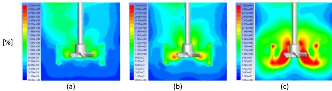
**Fig. 10.** Contour of turbulence intensity (%) at  $t = 20$  s (a) 46 rpm, (b) 81 rpm and (c) 165 rpm
