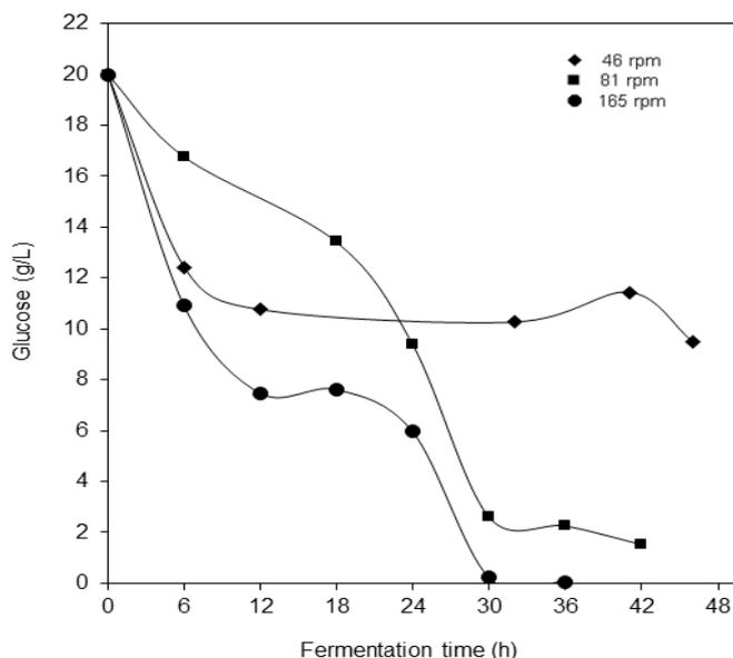
**Fig. 7.** Effect of stirring intensity on glucose consumption in hydrogen fermentation by *E. aerogenes* NBRC 13534
