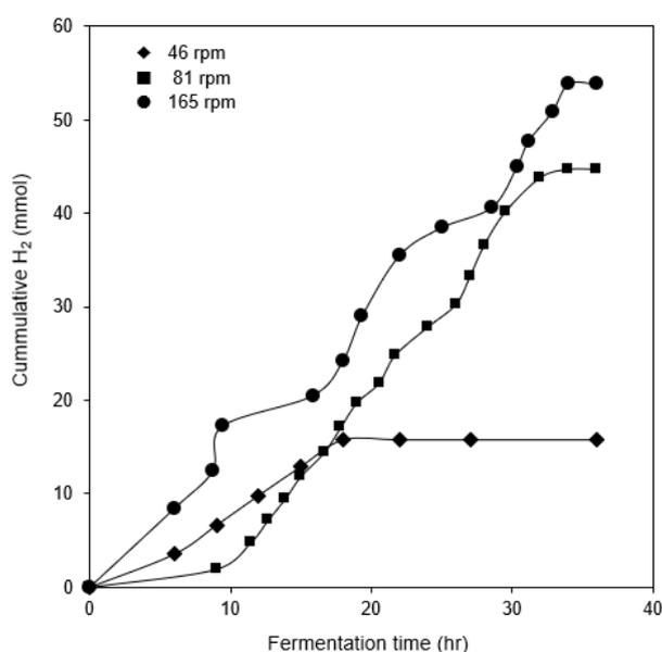
**Fig. 9.** Effect of stirring intensity on hydrogen produced in hydrogen fermentation by *E. aerogenes* NBRC 13534
