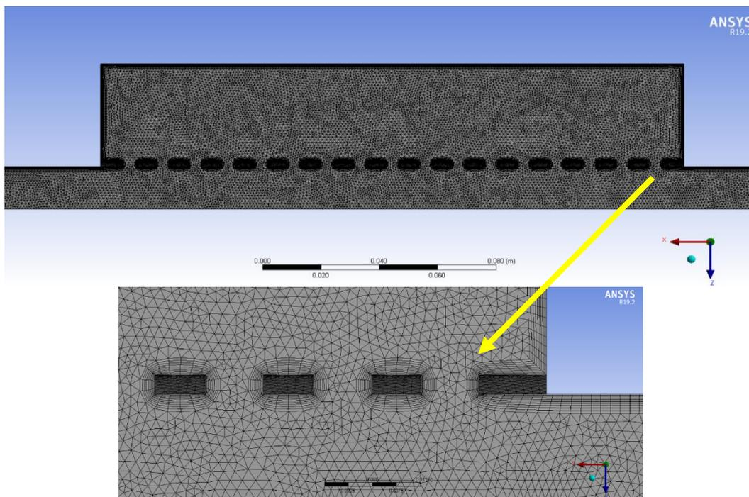
**Fig. 4.** The unstructured grid of the silencer model
