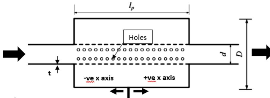
Fig. 1. Main construction of the silencer
