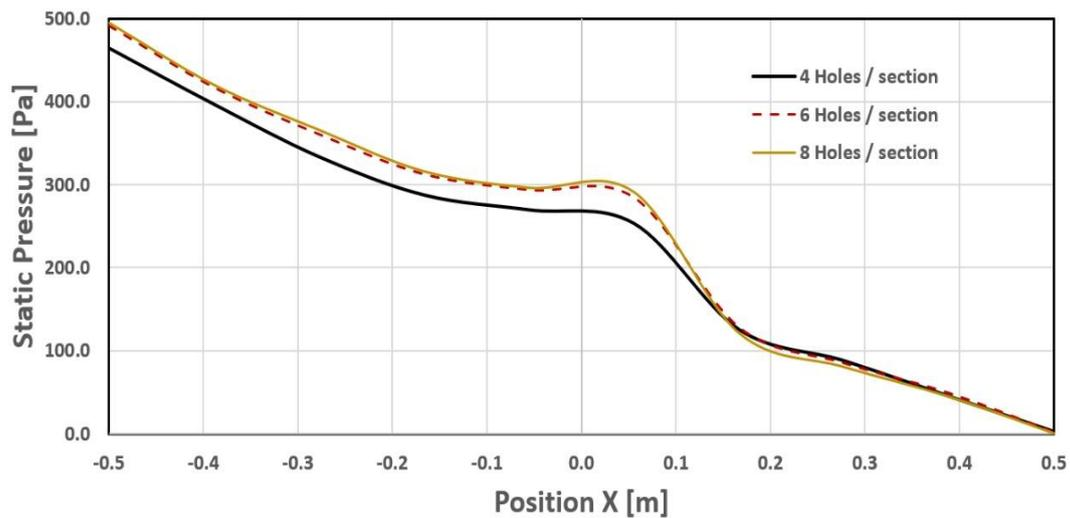
Fig. 9. Illustrating the effect of number of holes in transverse direction on pressure drop
