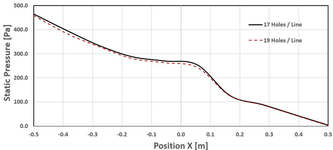
Fig. 10. Illustrating the effect of number of holes in longitudinal direction on pressure drop
