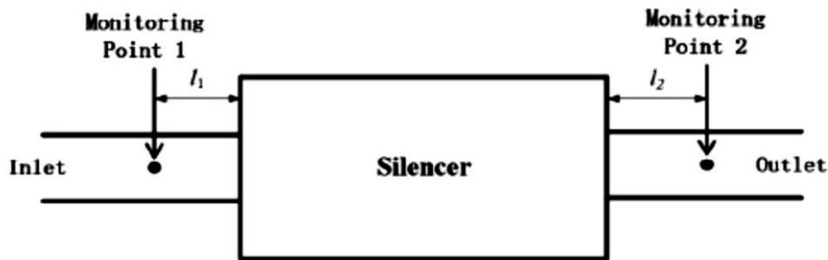
Fig. 1. Boundary of the model and location of the monitoring points
