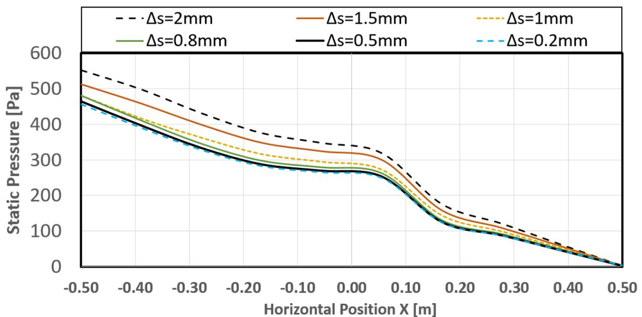
**Fig. 3.** Grid independency study ( $L=200\text{mm}$ , domain  $2L$ , total length of the model  $5L=1\text{m}$ )
