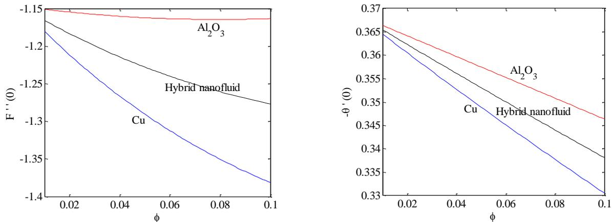
Fig. 9. Skin friction & Nusselt number for nanofluid and hybrid nanofluid
