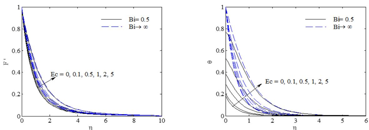
Fig. 4. Velocity & temperature profiles versus Eckert number  $Ec$
