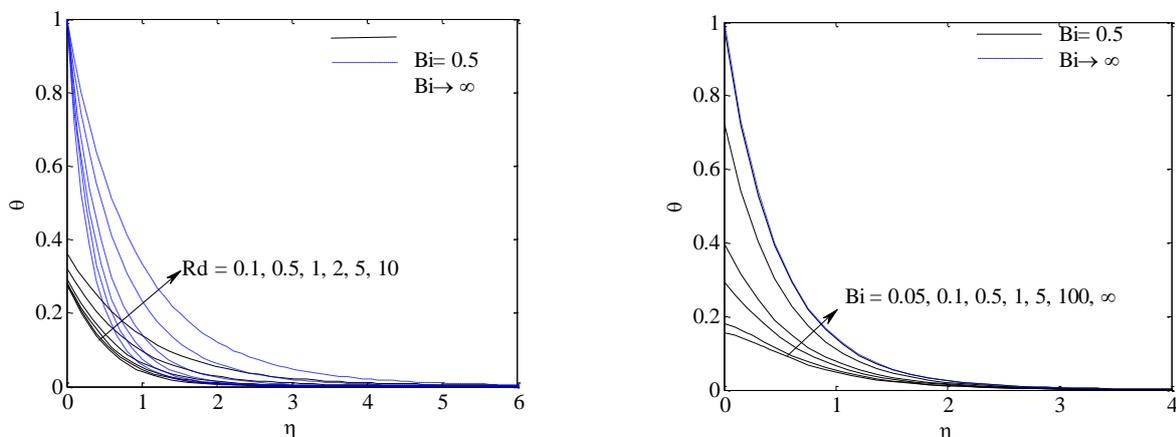
Fig. 5. Temperature curves versus radiation parameter and Biot number
