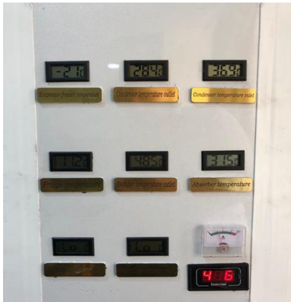
Fig. 8. The thermal sensor panel connected to the refrigerator parts
