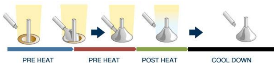
Fig. 4. Sequences of laser soldering process
