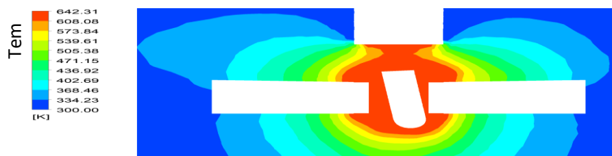
Fig. 6. Temperature distribution of simulated laser soldering process
