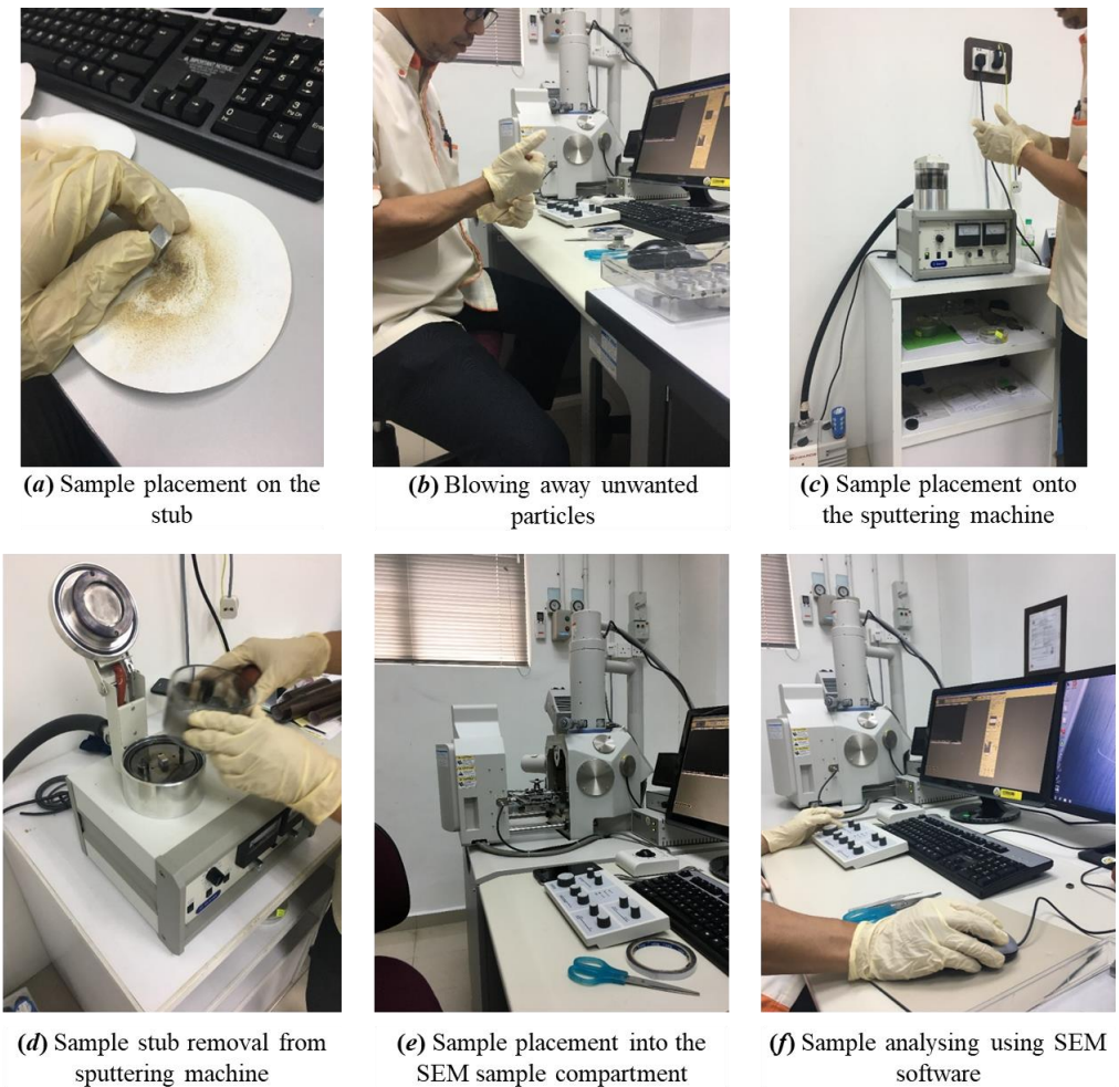
Fig. 1. General process flow of analysing the sediment sample using sputtering machine and scanning electronic microscope (SEM)
