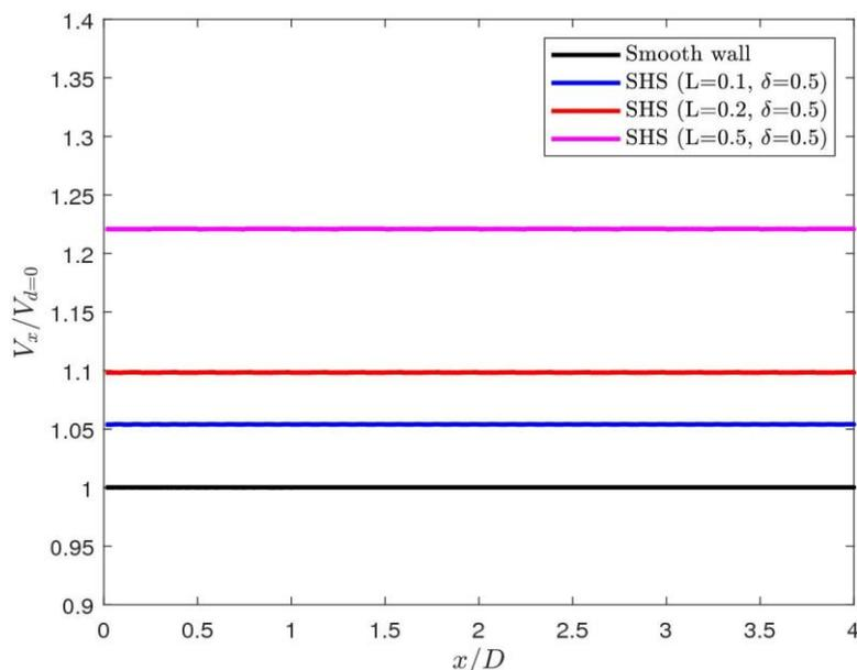
**Fig. 4.** Dimensionless averaged axial velocity for thermal flow scenarios considered
