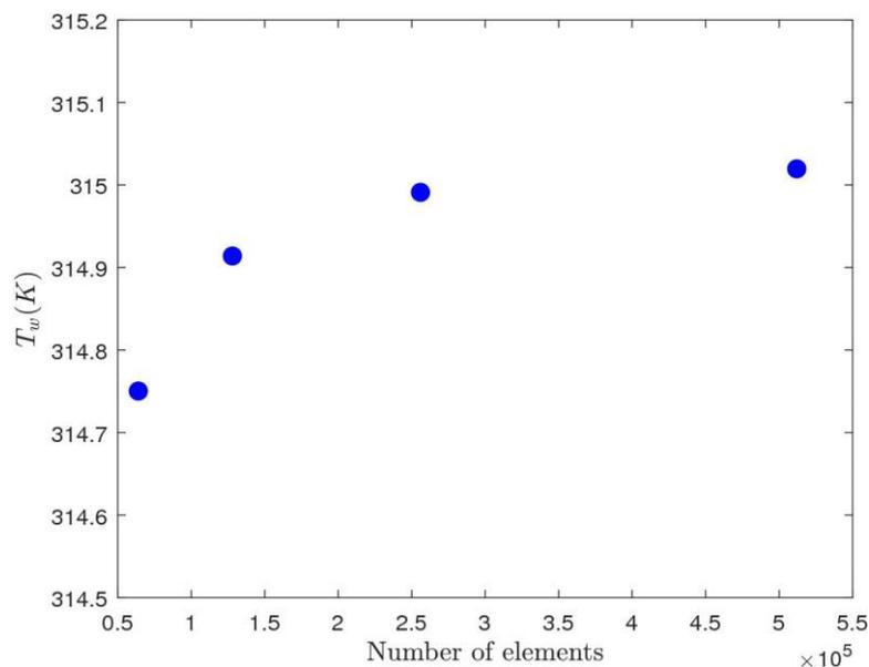
**Fig. 2.** Grid independence test for thermal flow over superhydrophobic transverse grooves with  $L = 0.1$  and  $\delta = 0.5$
