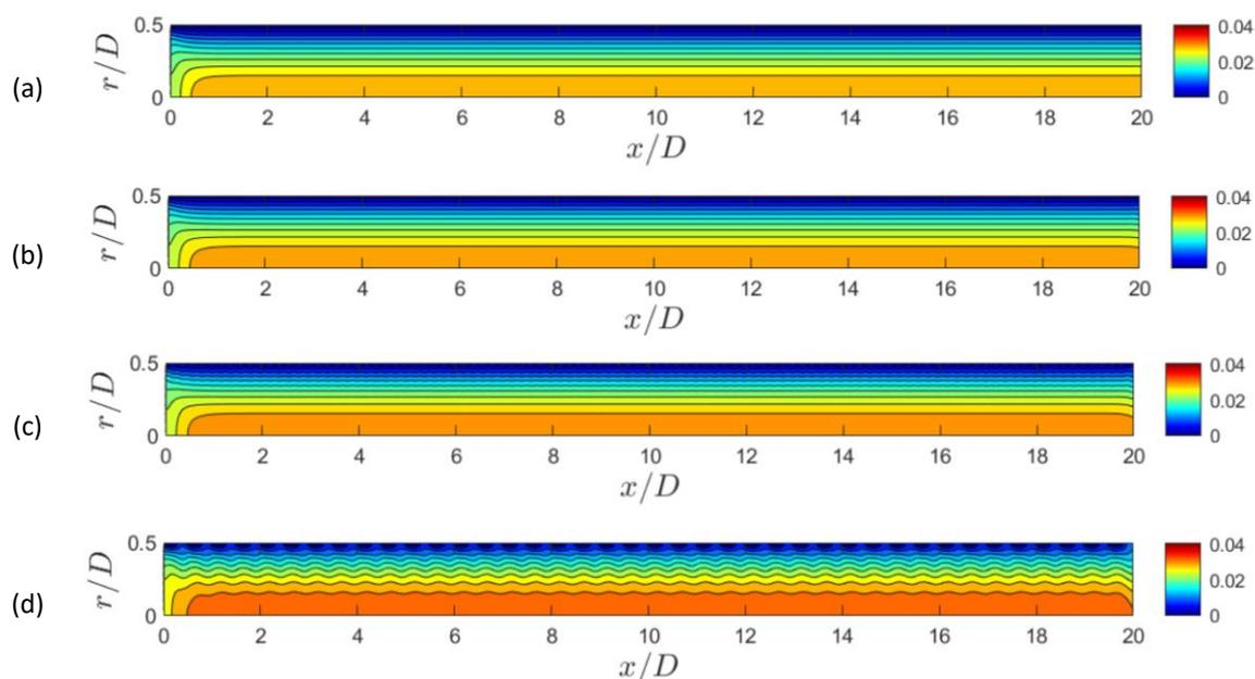
**Fig. 3.** Velocity fields for flow through tube having (a) smooth wall, superhydrophobic transverse grooves with (b)  $L = 0.1$  and  $\delta = 0.5$ , (c)  $L = 0.2$  and  $\delta = 0.5$ , and (d)  $L = 0.5$  and  $\delta = 0.5$
