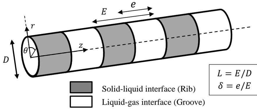
**Fig. 1.** Schematic of a tube patterned with superhydrophobic transverse grooves
