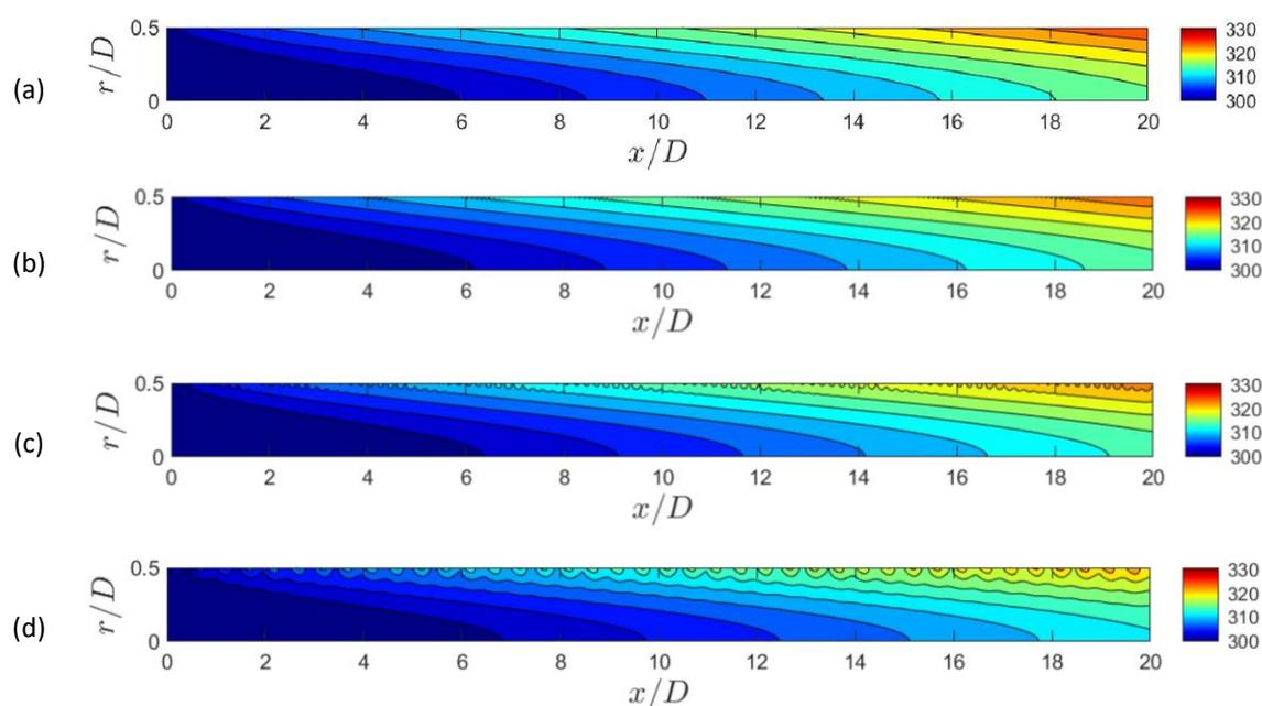
**Fig. 6.** Temperature fields for thermal flow through tube having (a) smooth wall, superhydrophobic transverse grooves with (b)  $L = 0.1$  and  $\delta = 0.5$ , (c)  $L = 0.2$  and  $\delta = 0.5$ , and (d)  $L = 0.5$  and  $\delta = 0.5$
