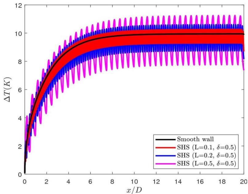
Fig. 8. Temperature difference for thermal flow scenarios considered
