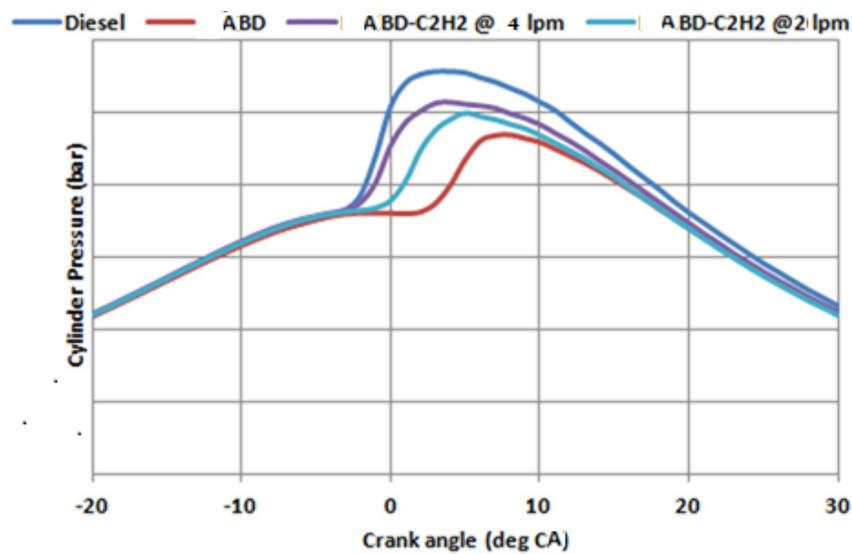
Fig. 8. Highest pressure variation per crank angle at maximum capacity
