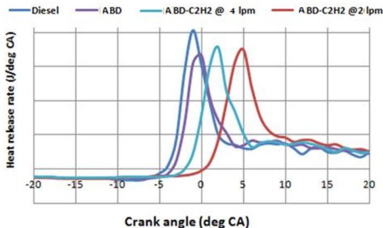
Fig. 9. HRR variation per crank angle at maximum capacity
