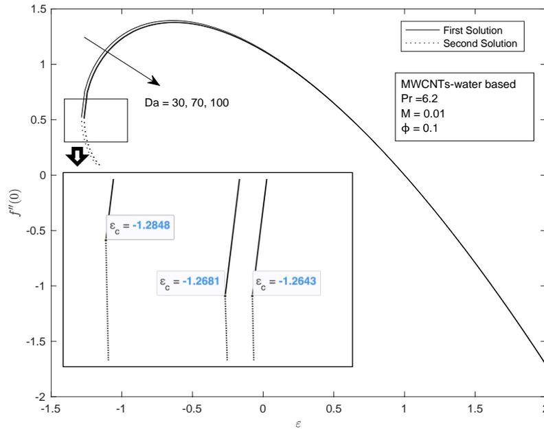
**Fig. 4.** Variation of  $f''(0)$  with different  $Da$  and  $\varepsilon$  for MWCNT-water based
