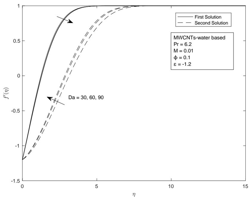
**Fig. 7.** Effect of different values of  $Da$  on the velocity profile using various  $\eta$  and for MWCNT-water based
