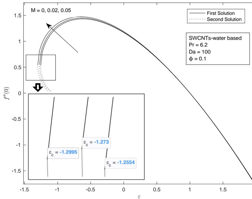
**Fig. 2.** Variation of  $f''(0)$  with different  $M$  and  $\varepsilon$  for SWCNT- water based
