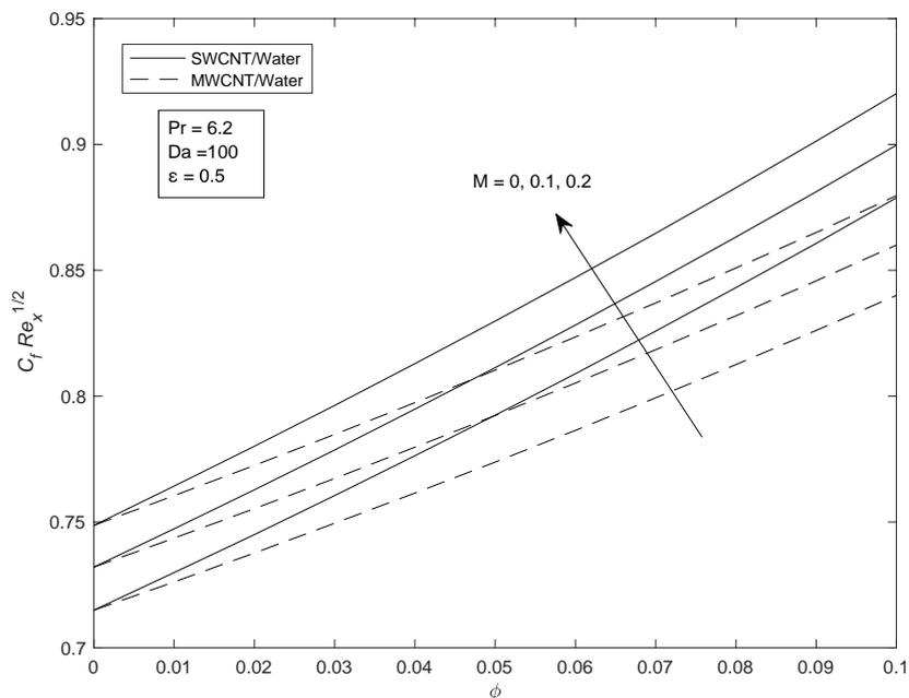
**Fig. 10.** Effect of different values of  $M$  on the skin friction coefficient using various  $\phi$  for SWCNT-water based and MWCNT-water based
