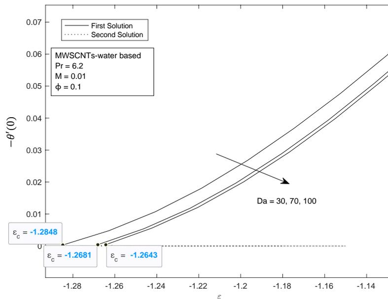
**Fig. 5.** Variation of  $-\theta'(0)$  with different  $Da$  and  $\varepsilon$  for MWCNT-water based
