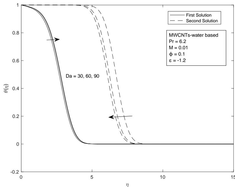
**Fig. 9.** Effect of different values of  $Da$  on the temperature profile using various  $\eta$  and for MWCNT-water based
