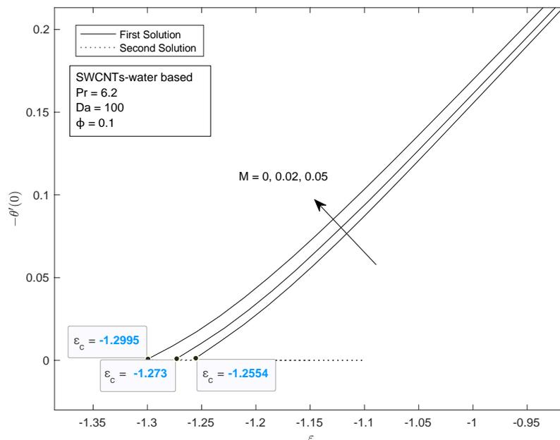
**Fig. 3.** Variation of  $-\theta'(0)$  with different  $M$  and  $\varepsilon$  for SWCNT- water based
