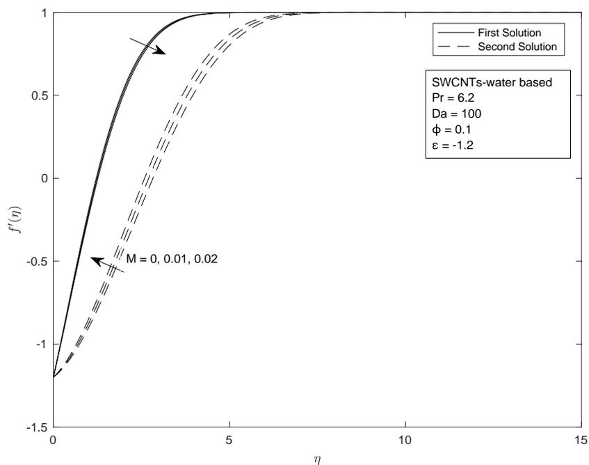
**Fig. 6.** Effect of different values of  $M$  on the velocity profile using various  $\eta$  and for SWCNT-water based
