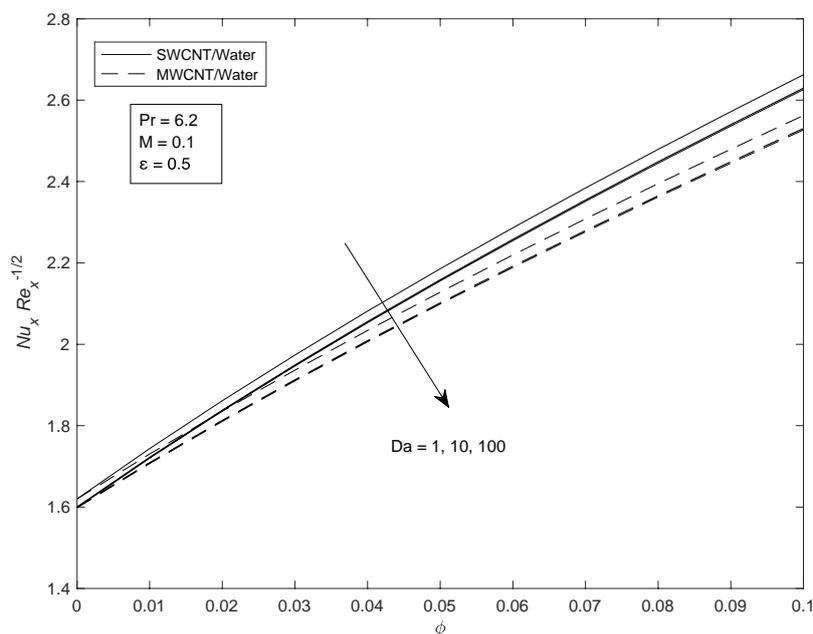
**Fig. 11.** Effect of different values of  $Da$  on the Nusselt Number using various  $\phi$  for SWCNT-water based and MWCNT-water based
