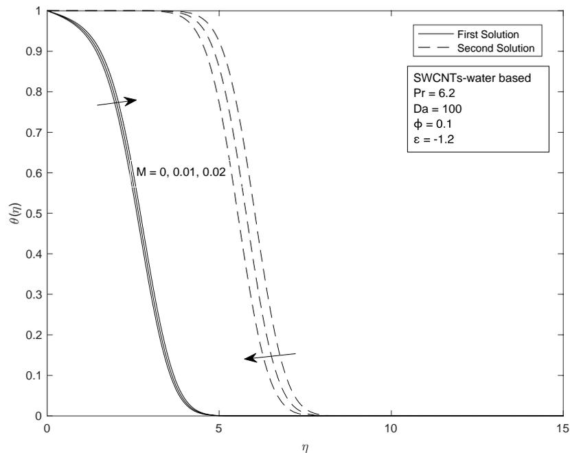
**Fig. 8.** Effect of different values of  $M$  on the temperature profile using various  $\eta$  and for SWCNT-water based
