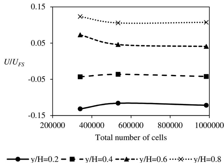
**Figure 3:** Streamwise velocity along the vertical middle of street canyon under different thermal flow conditions
