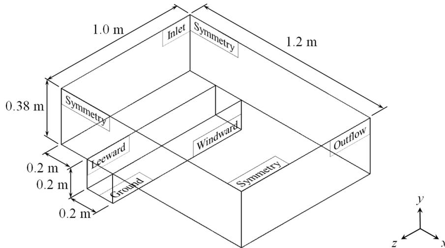
**Figure 2:** Schematic diagram of the computational domain and boundary conditions
