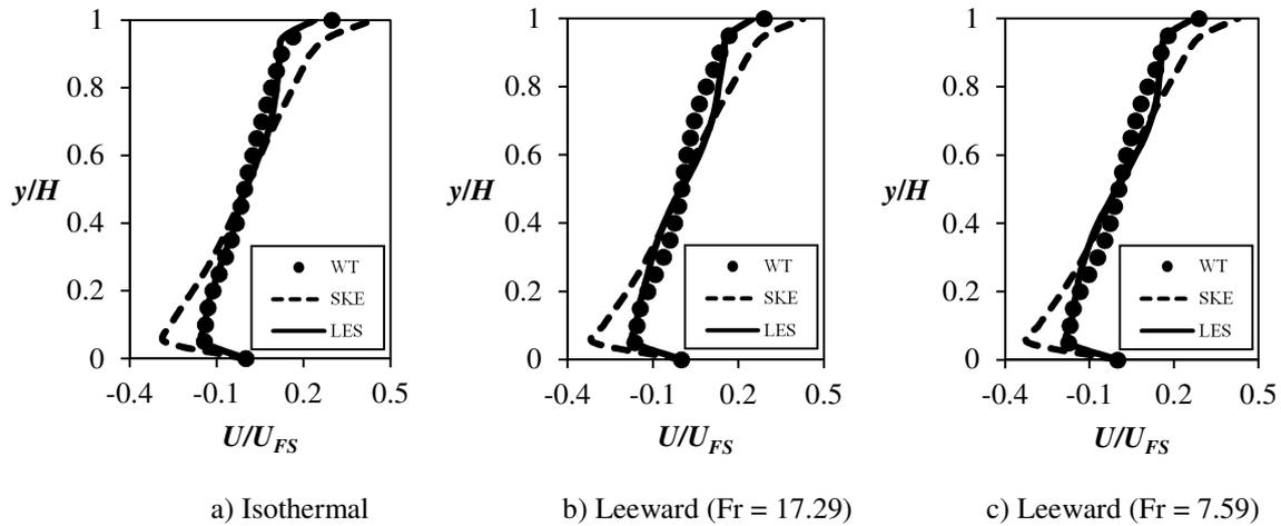
**Figure 4:** Normalized streamwise velocity along the vertical middle of street canyon under different thermal flow conditions
