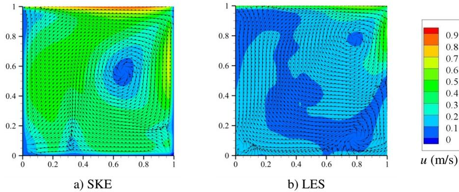
**Figure 5:** Contour and vector plot of velocity magnitude of windward wall heated at  $Fr = 7.59$
