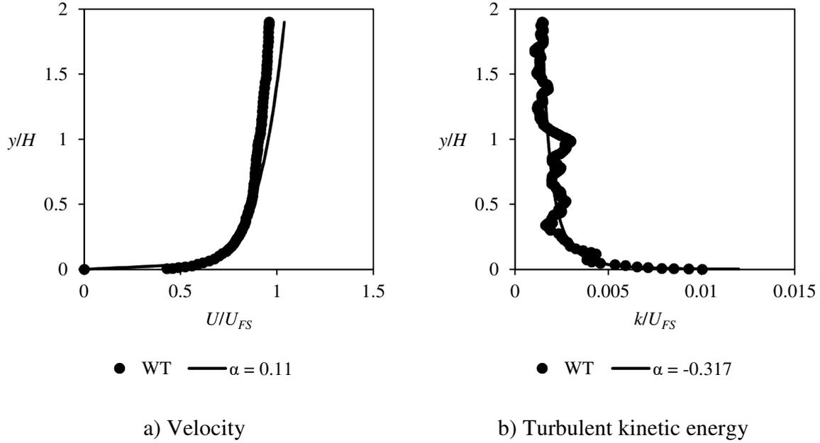
**Figure 1:** The variation of mean wind velocities with height from WT and from estimation using exponential law
