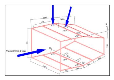
Figure 1: 3-D view of the combustor simulator
