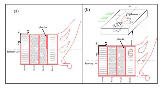
Figure 2: Location of the measurement planes (a) baseline case (b) compound case
