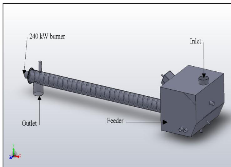
**Figure 1:**Schematic of the thermal dryer
