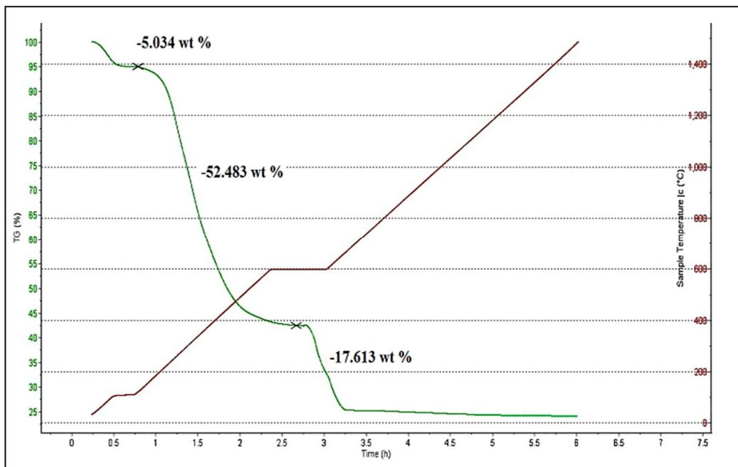
**Figure 4:**TGA results for sewage sludge
