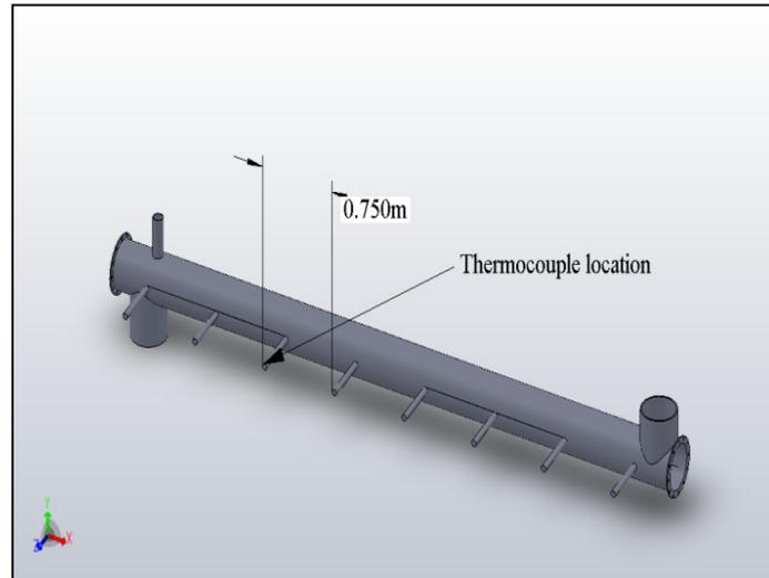
**Figure 2:** Thermocouple location along the dryer
