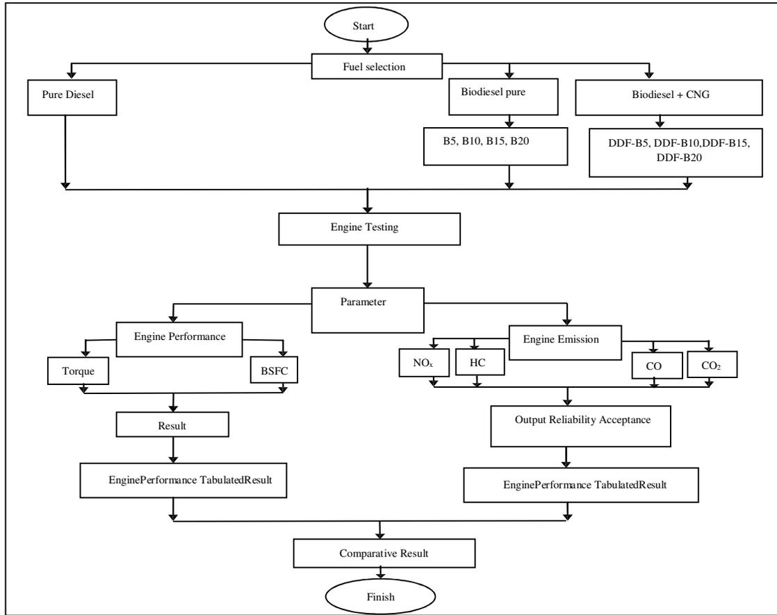
**Figure 1:** Flow chart of the entire step of experiment
