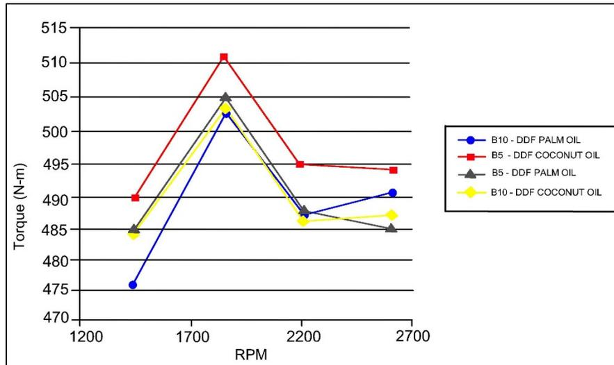
**Figure 2:** Torque against engine speed (RPM) for various blends of biodiesel-natural gas
