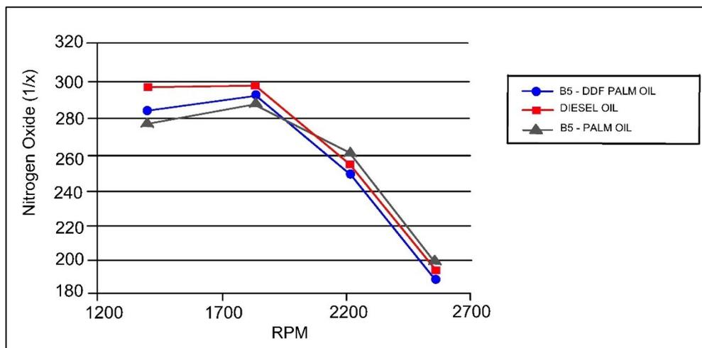
**Figure 11:** Nitrogen oxide against engine speed (RPM) for various fuels
