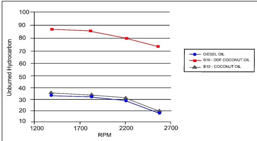
**Figure 13:** Unburned hydrocarbon emission against engine speed (RPM) for various fuels
