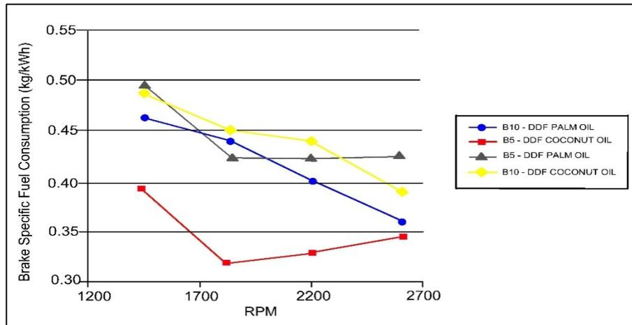
**Figure 4:** Brake specific fuel consumption against engine speed (RPM) for various blend biodiesel-natural gas
