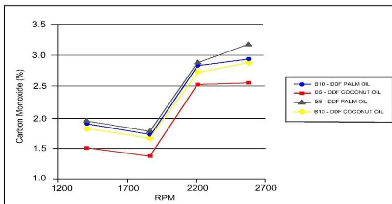
**Figure 8:** Carbon monoxide against engine speed (RPM) for various blends of biodiesel-natural gas
